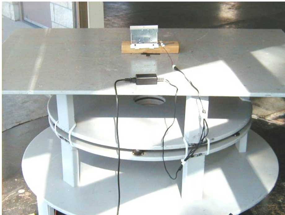
Radiated Emissions Test Configuration
