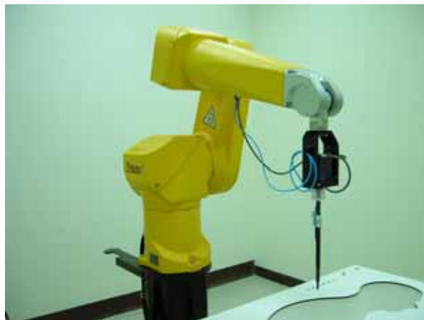
Fig. 5.2 Probe setup on robot
