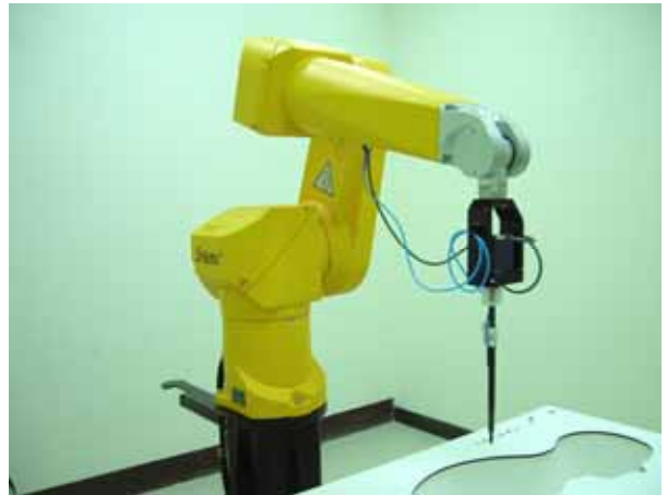
Fig. 5.2 Probe setup on robot
