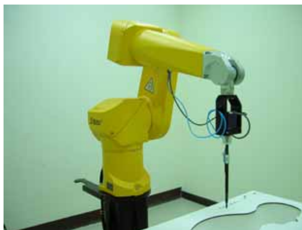
Fig. 5.2 Probe setup on robot
