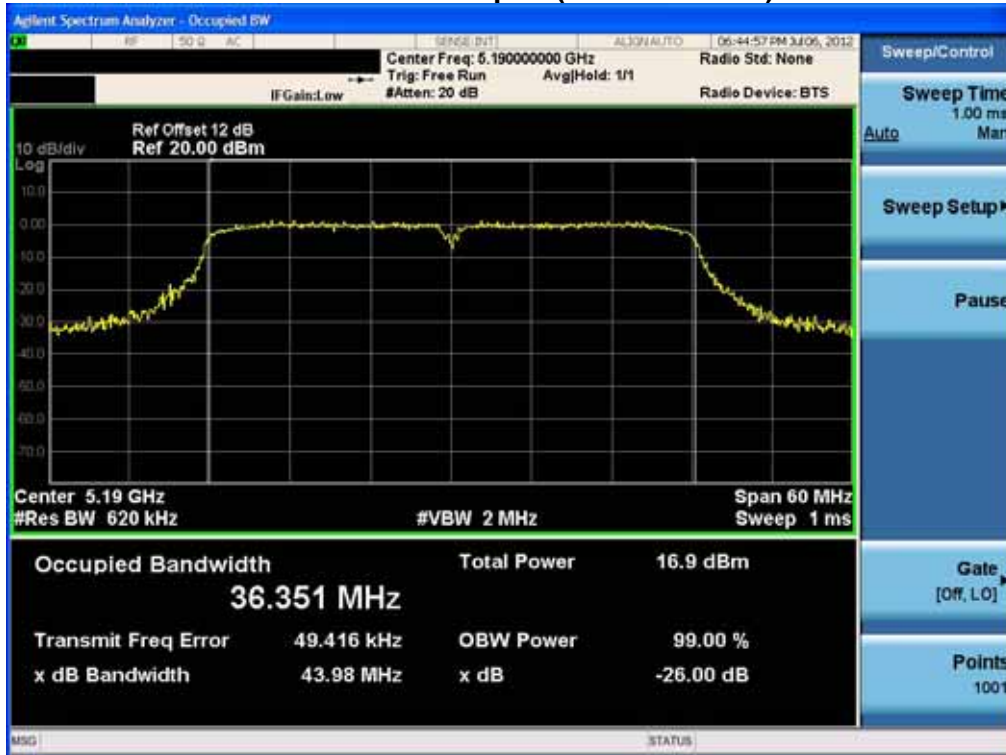
26 dB Bandwidth plot (802.11n-CH 46)
