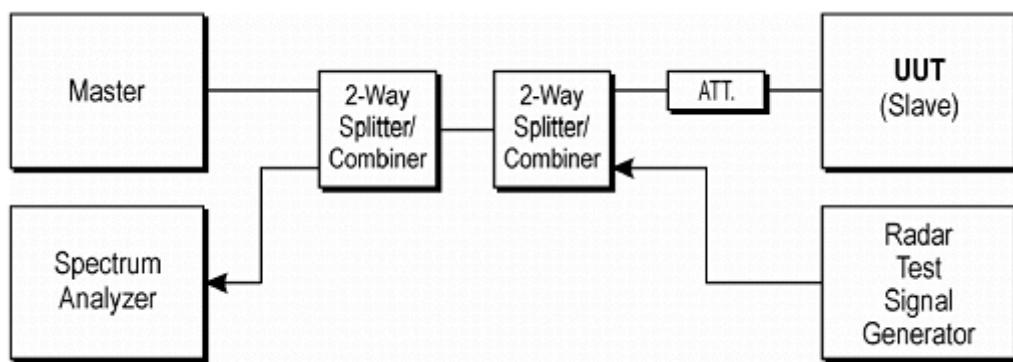
**Figure 3-1. Conducted Test Setup for DFS**
