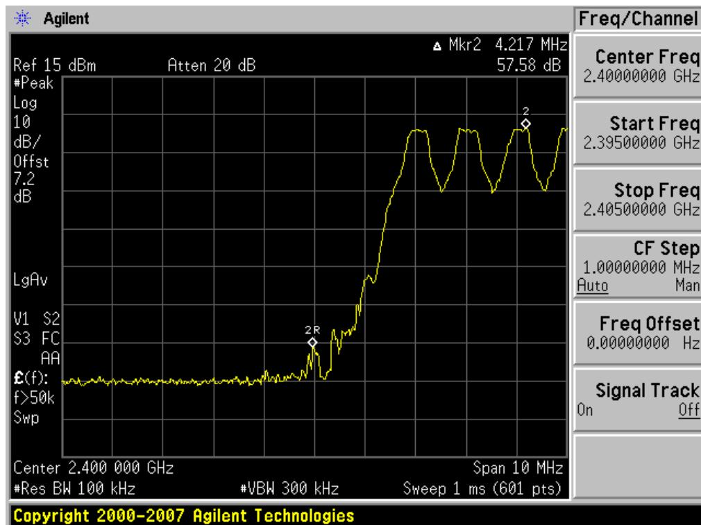
Test Plots with hopping (GFSK)
