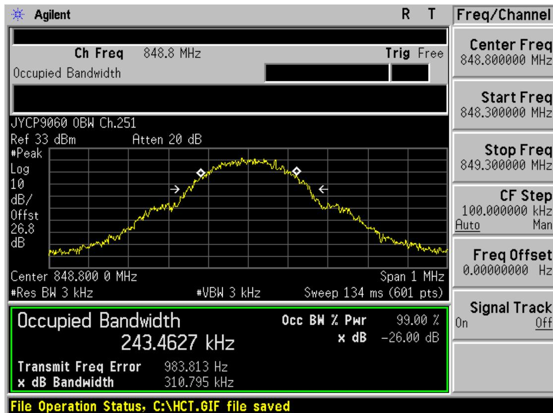
■ GSM850 EDGE (128 CH.) Occupied Bandwidth
