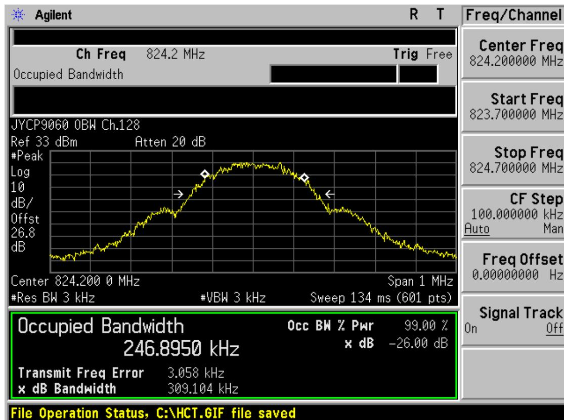
■ GSM850 MODE (190 CH.) Occupied Bandwidth
