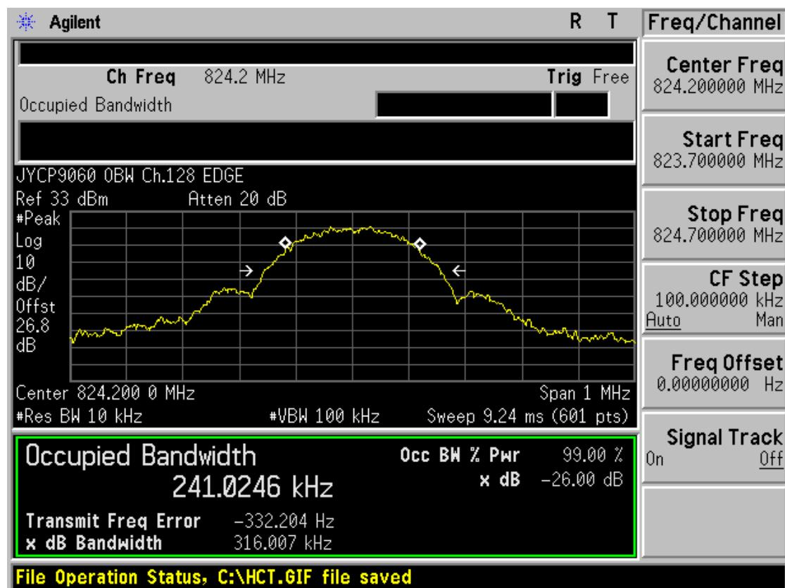
■ GSM1900 MODE (512 CH.) Occupied Bandwidth
