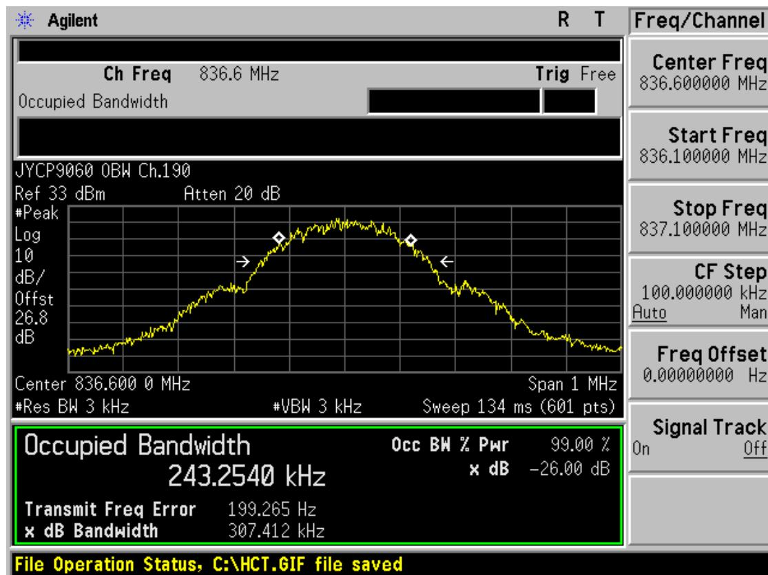
■ GSM850 MODE (251 CH.) Occupied Bandwidth
