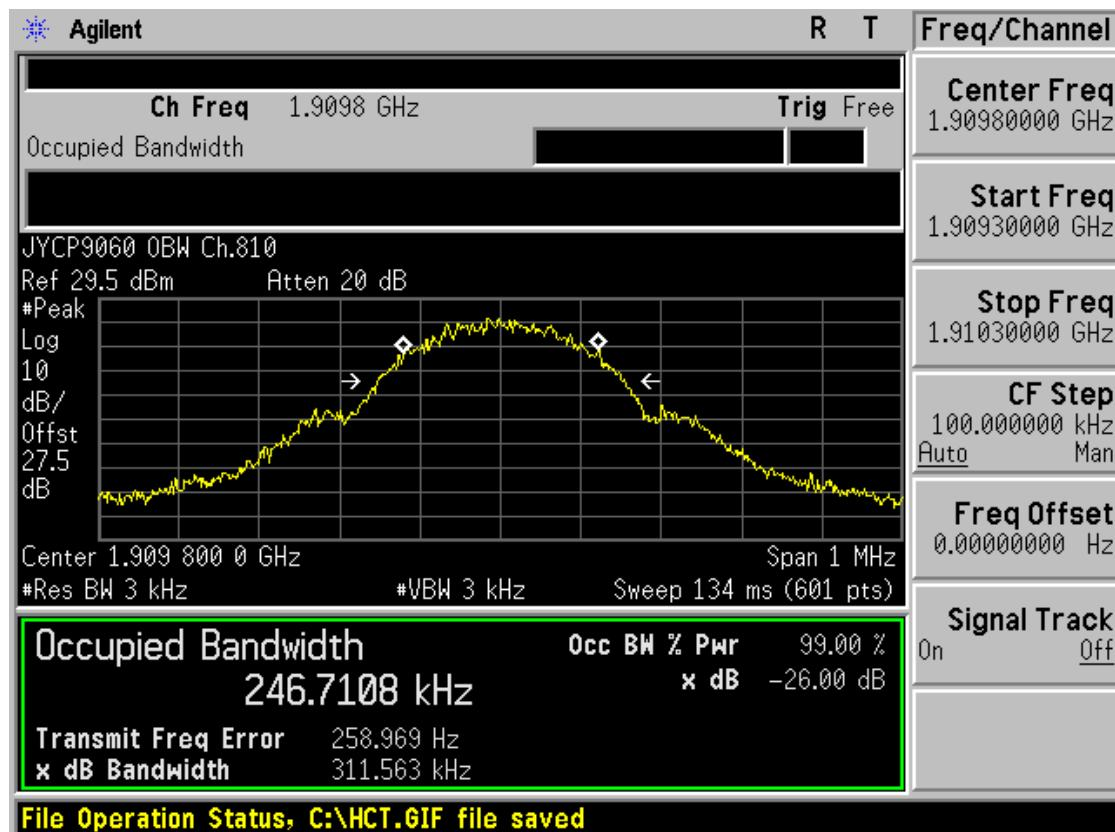
■ GSM1900 EDGE (661 CH.) Occupied Bandwidth
