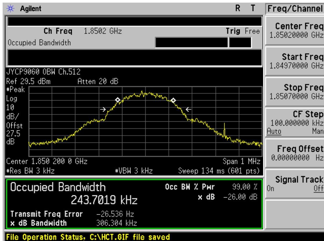
■ GSM1900 MODE (661 CH.) Occupied Bandwidth
