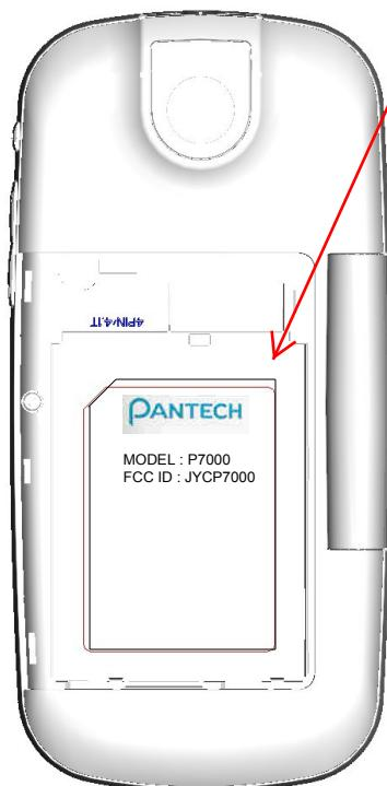
Battery compartment. Label located below the battery pack. Product is provided without the battery pack installed, so the user can see the label at the time of purchase.
