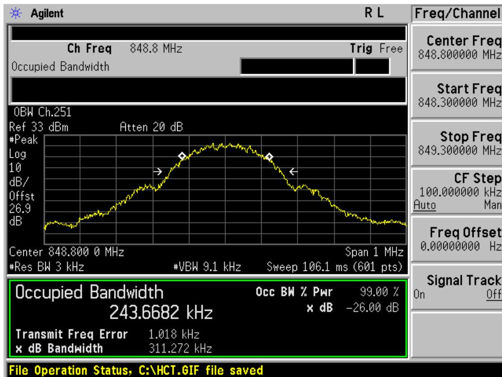
■ GSM850 EDGE (128 CH.) Occupied Bandwidth
