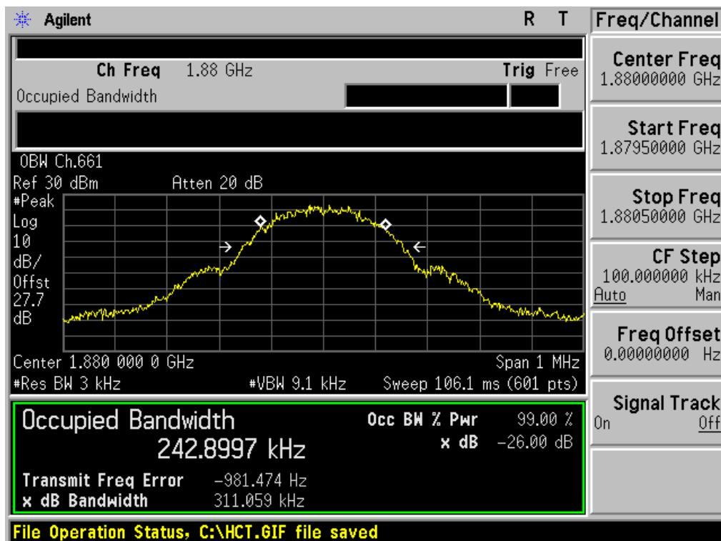
■ GSM1900 MODE (810 CH.) Occupied Bandwidth
