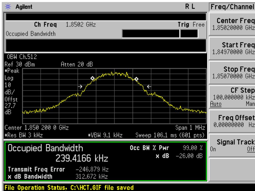
■ GSM1900 MODE (661 CH.) Occupied Bandwidth
