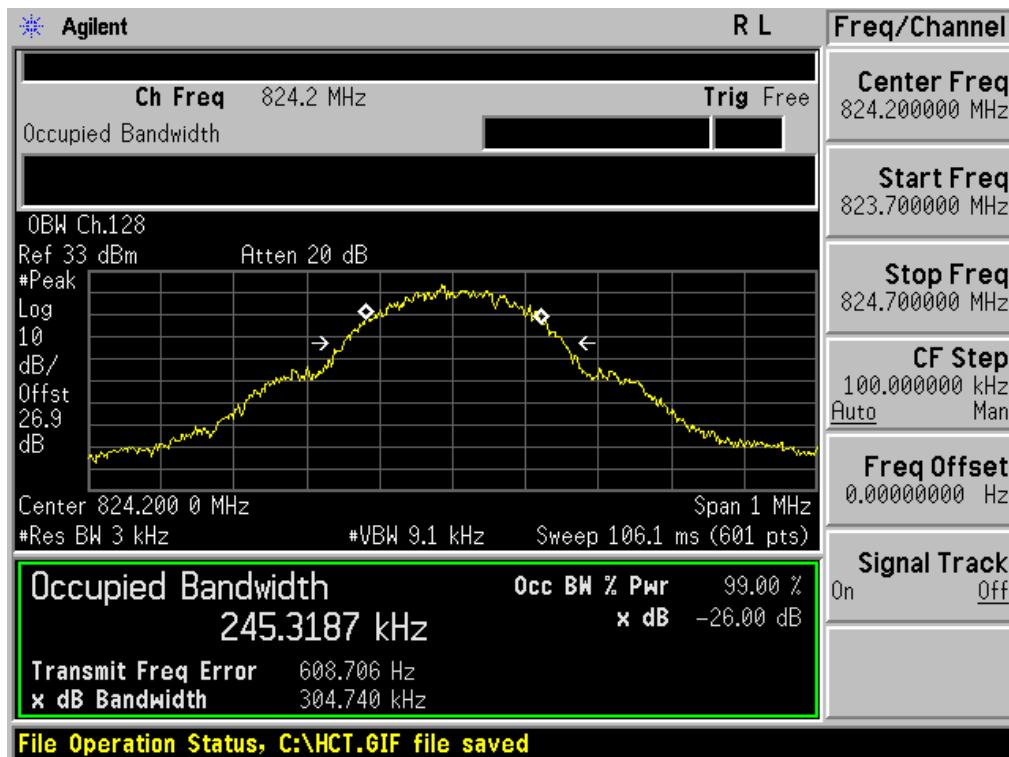
■ GSM850 MODE (190 CH.) Occupied Bandwidth
