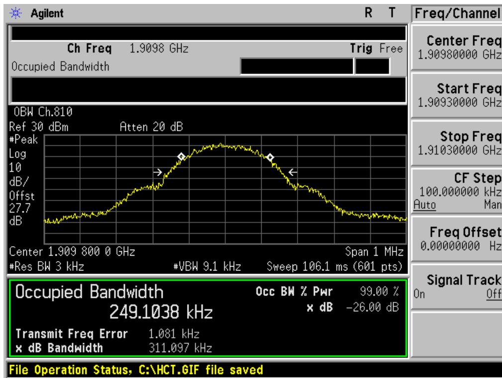
■ GSM1900 EDGE (810 CH.) Occupied Bandwidth
