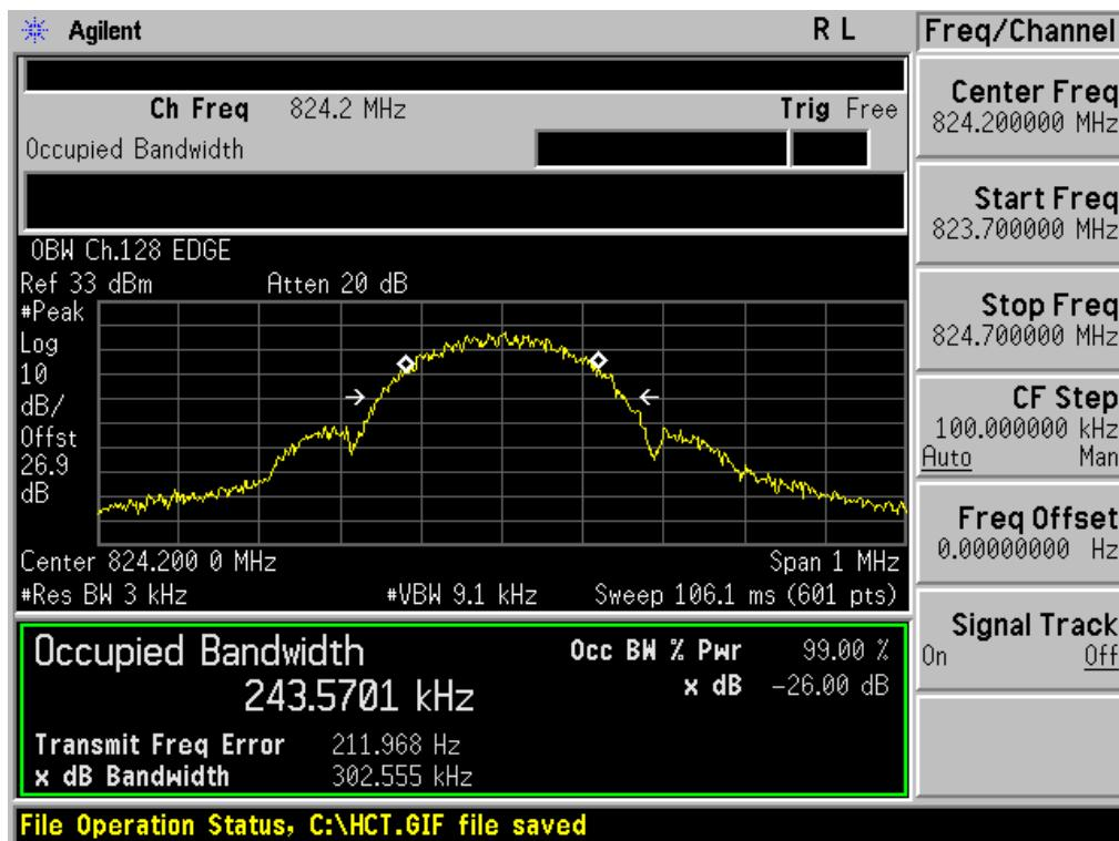
■ GSM1900 MODE (512 CH.) Occupied Bandwidth
