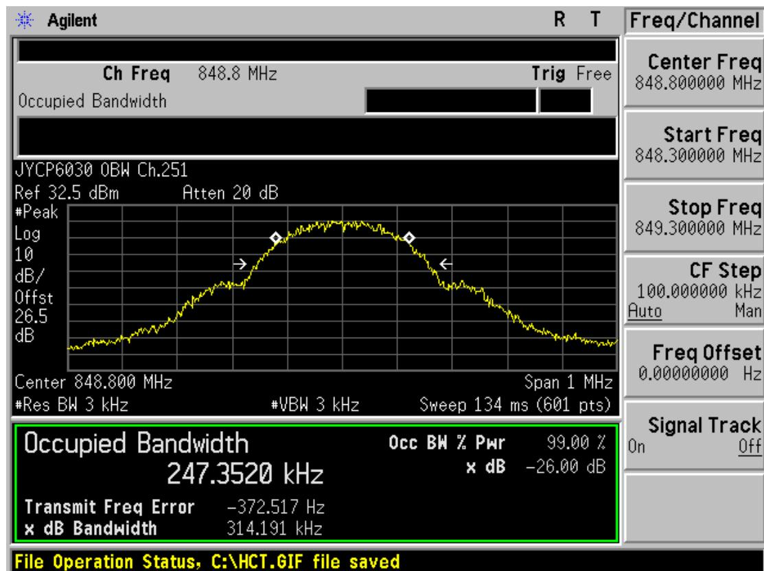
■ GSM850 EDGE (190 CH.) Occupied Bandwidth
