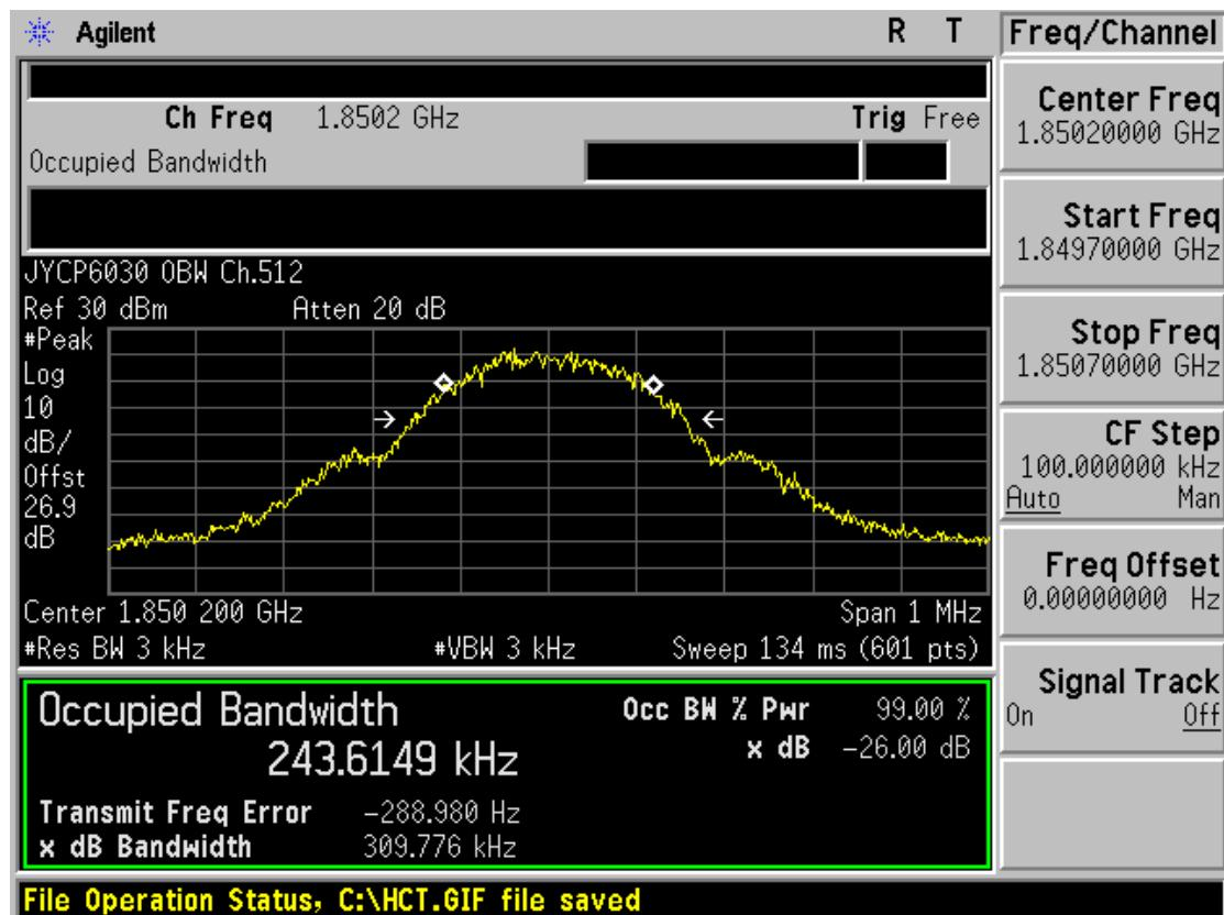
■ GSM1900 MODE (661 CH.) Occupied Bandwidth
