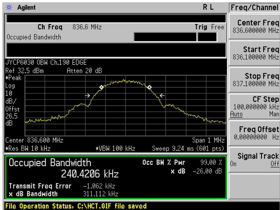
■ GSM1900 MODE (512 CH.) Occupied Bandwidth
