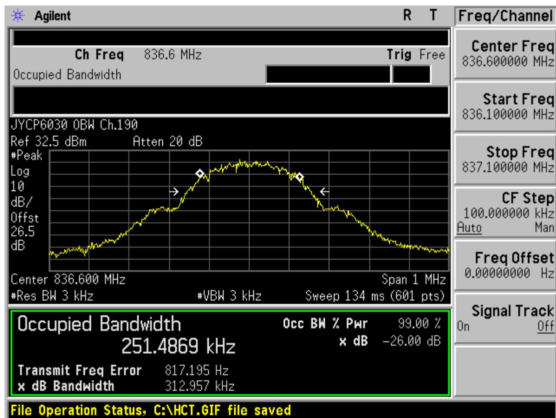
■ GSM850 MODE (251 CH.) Occupied Bandwidth
