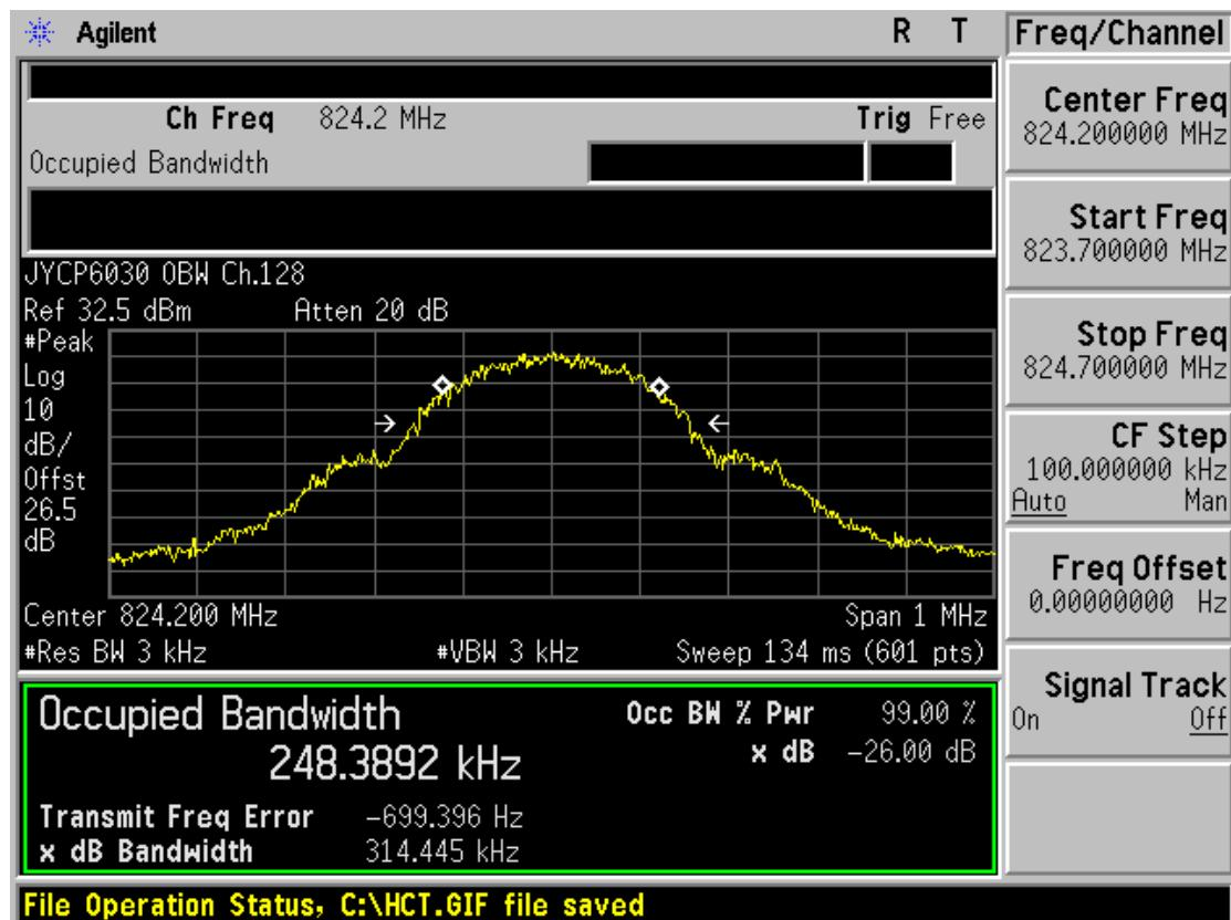
■ GSM850 MODE (190 CH.) Occupied Bandwidth
