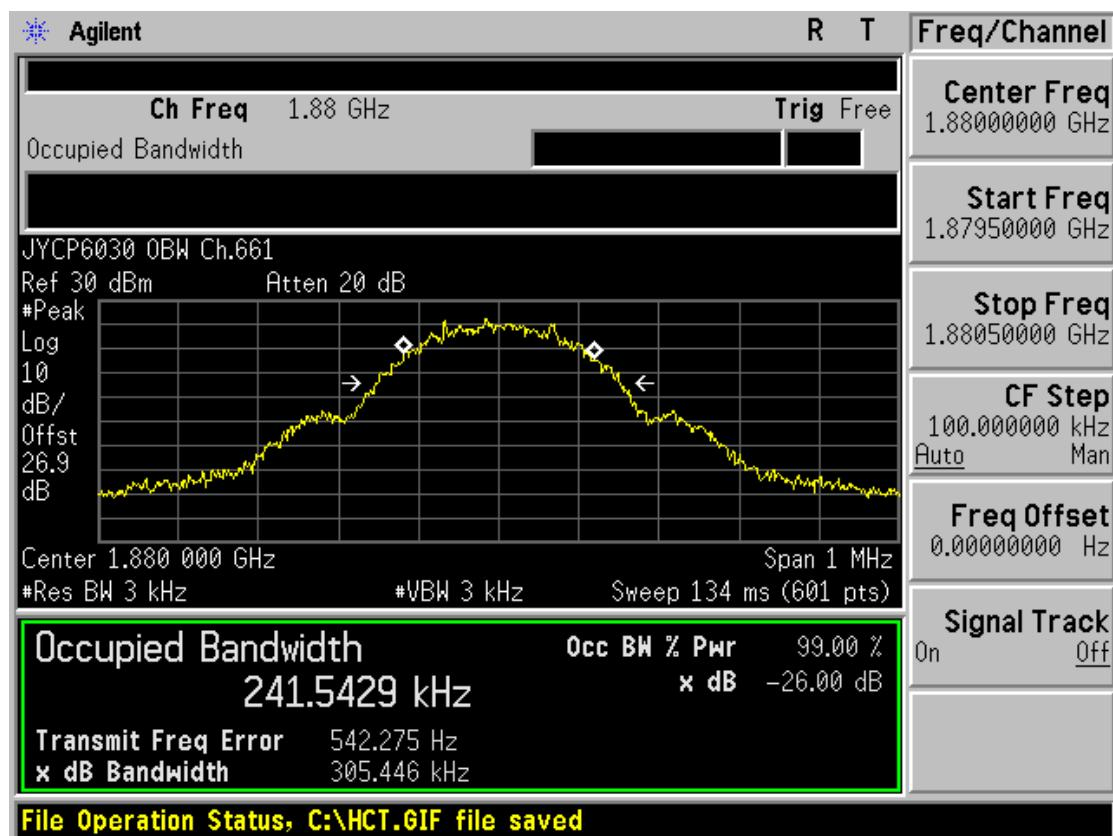
■ GSM1900 MODE (810 CH.) Occupied Bandwidth
