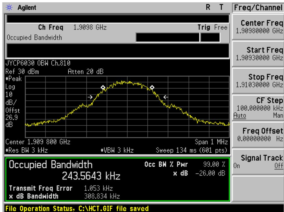
■ GSM1900 EDGE (512 CH.) Occupied Bandwidth
