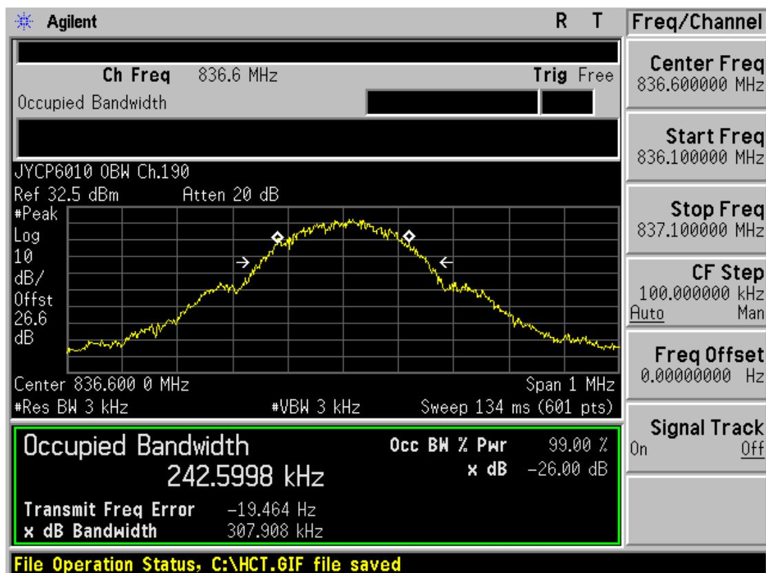
■ GSM850 MODE (251 CH.) Occupied Bandwidth
