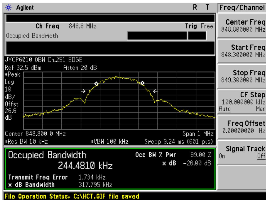
■ GSM1900 MODE (512 CH.) Occupied Bandwidth
