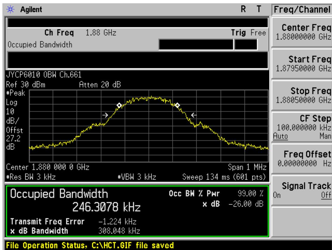
■ GSM1900 MODE (810 CH.) Occupied Bandwidth
