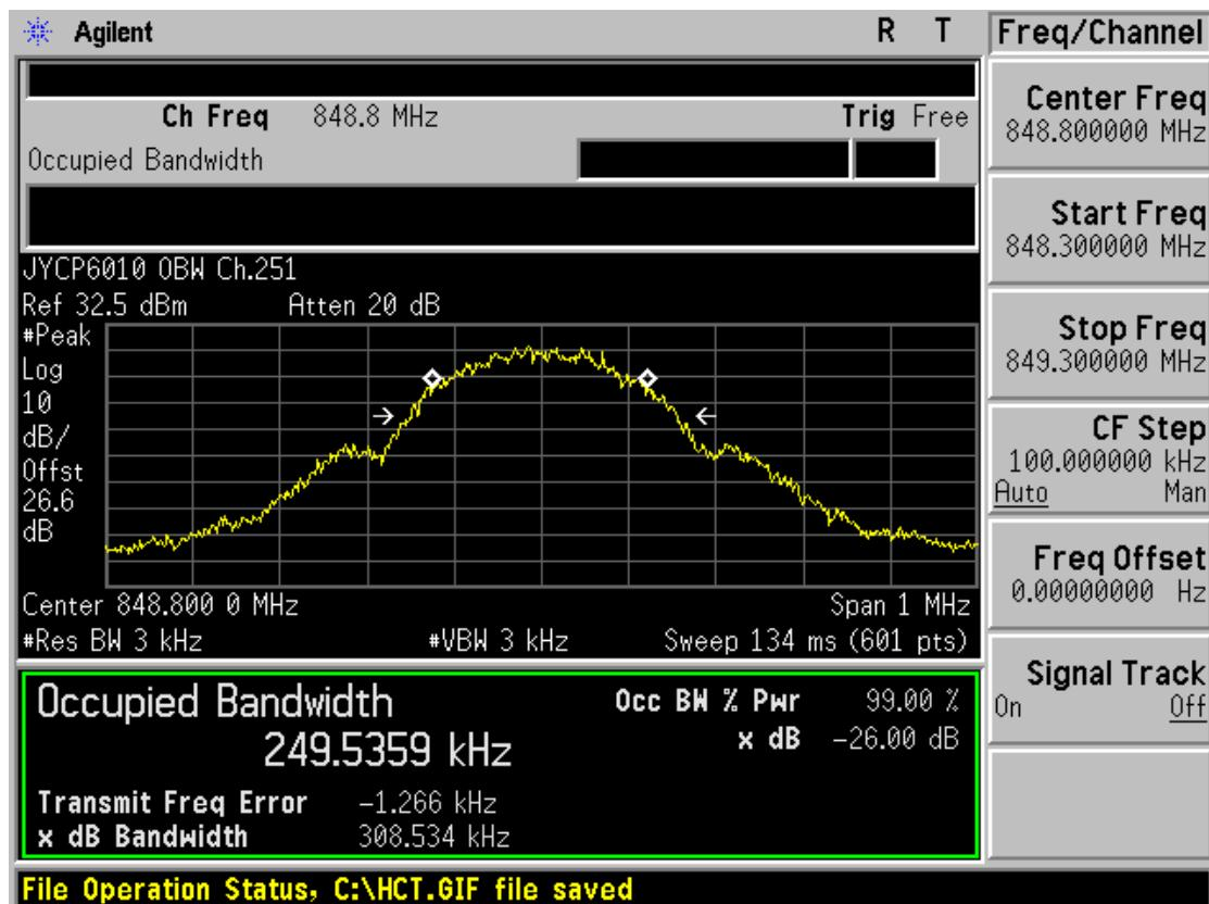
■ GSM850 EDGE (251 CH.) Occupied Bandwidth
