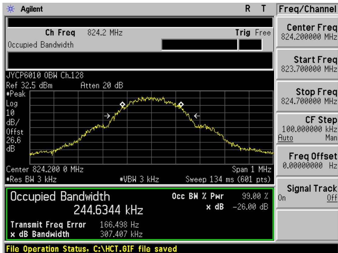
■ GSM850 MODE (190 CH.) Occupied Bandwidth
