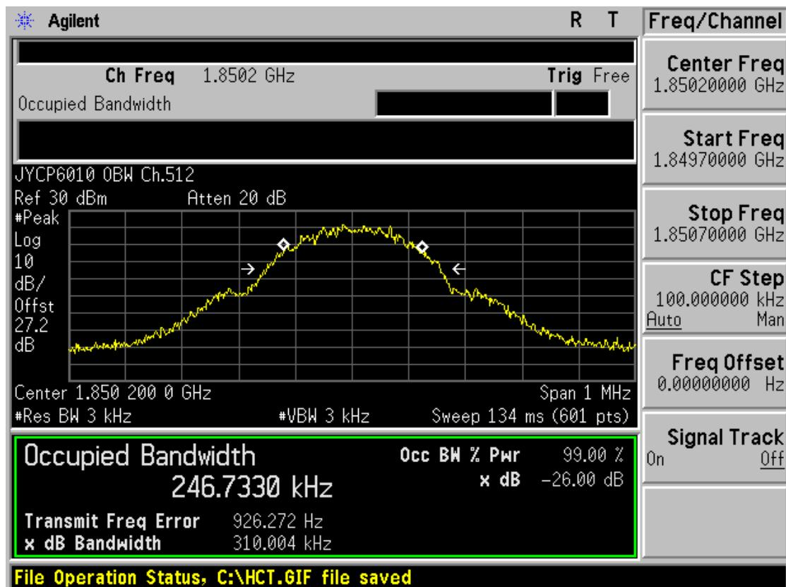
■ GSM1900 MODE (661 CH.) Occupied Bandwidth
