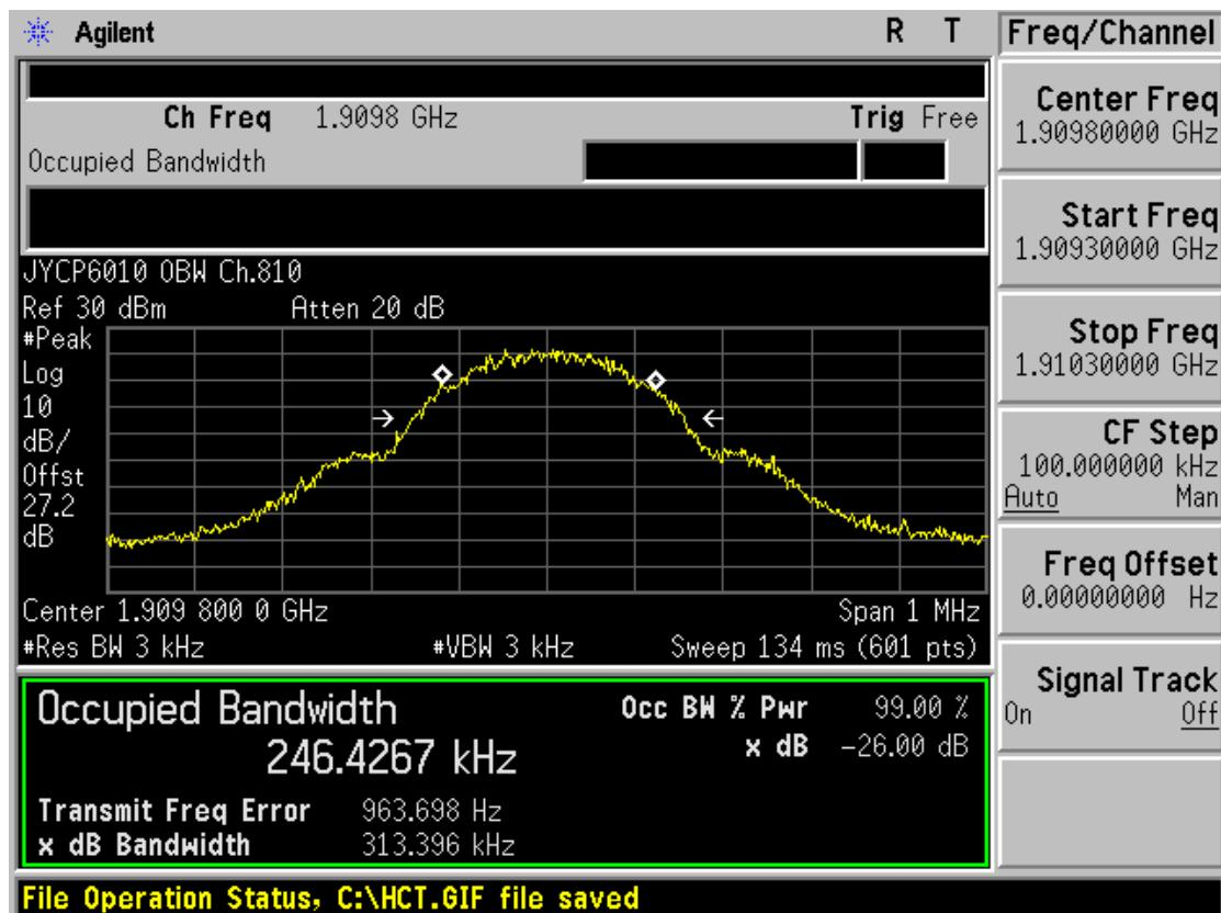
■ GSM1900 EDGE (512 CH.) Occupied Bandwidth
