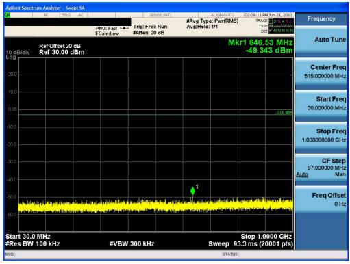
Test Plots (8DPSK) - 30 MHz - 1 GHz Spurious Emission (High-CH)
