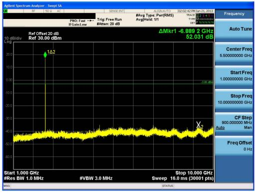
Test Plots (8DPSK) - 1 GHz - 10 GHz Spurious Emission (High-CH)
