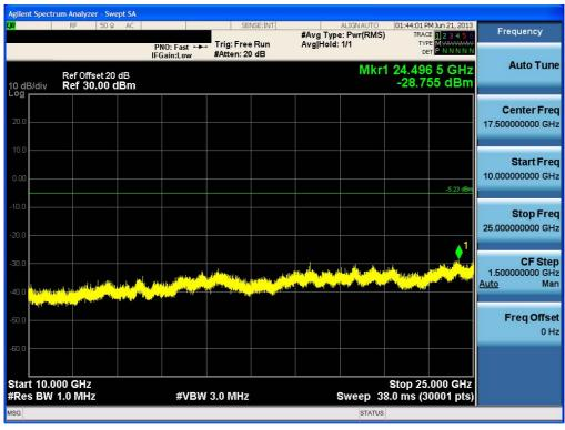
Test Plots (GFSK) - 10 GHz - 25 GHz Spurious Emission (Mid-CH)
