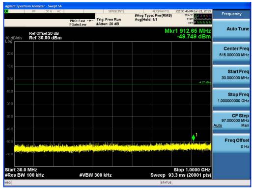
Test Plots (8DPSK) - 30 MHz - 1 GHz Spurious Emission (Low-CH)
