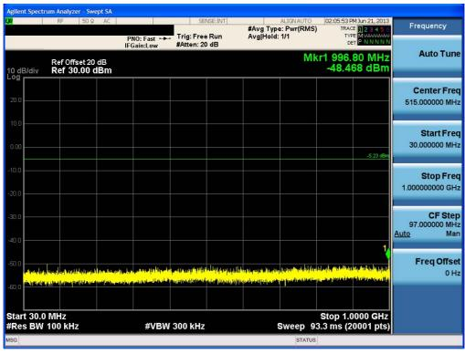
Test Plots (GFSK) - 30 MHz - 1 GHz Spurious Emission (Mid-CH)
