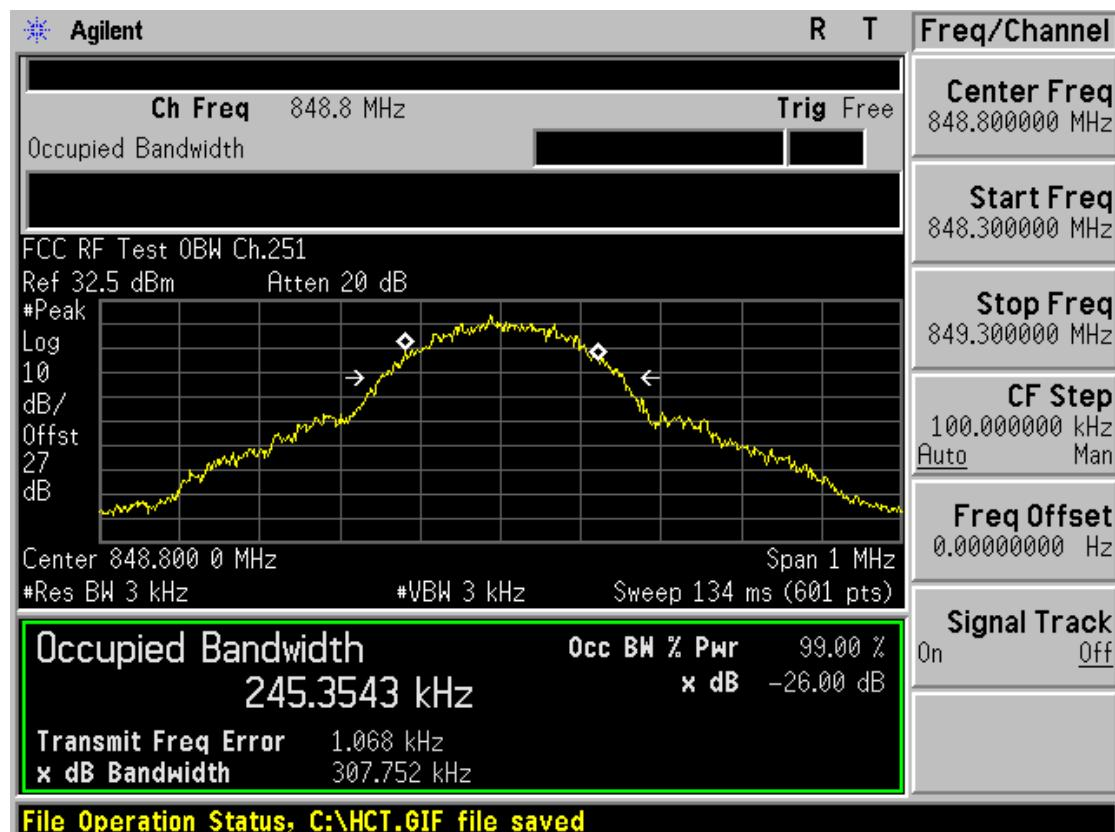
■ GSM850 EDGE (128 CH.) Occupied Bandwidth
