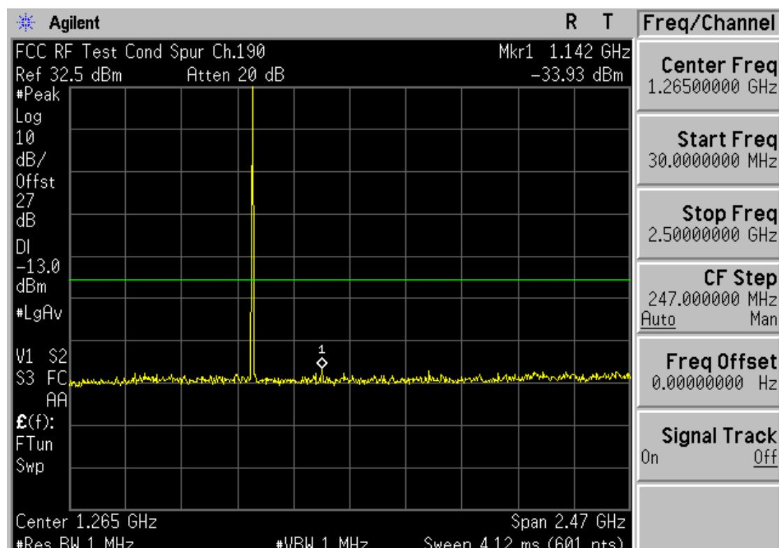
■ GSM850 MODE (190 CH.) Conducted Spurious Emissions2
