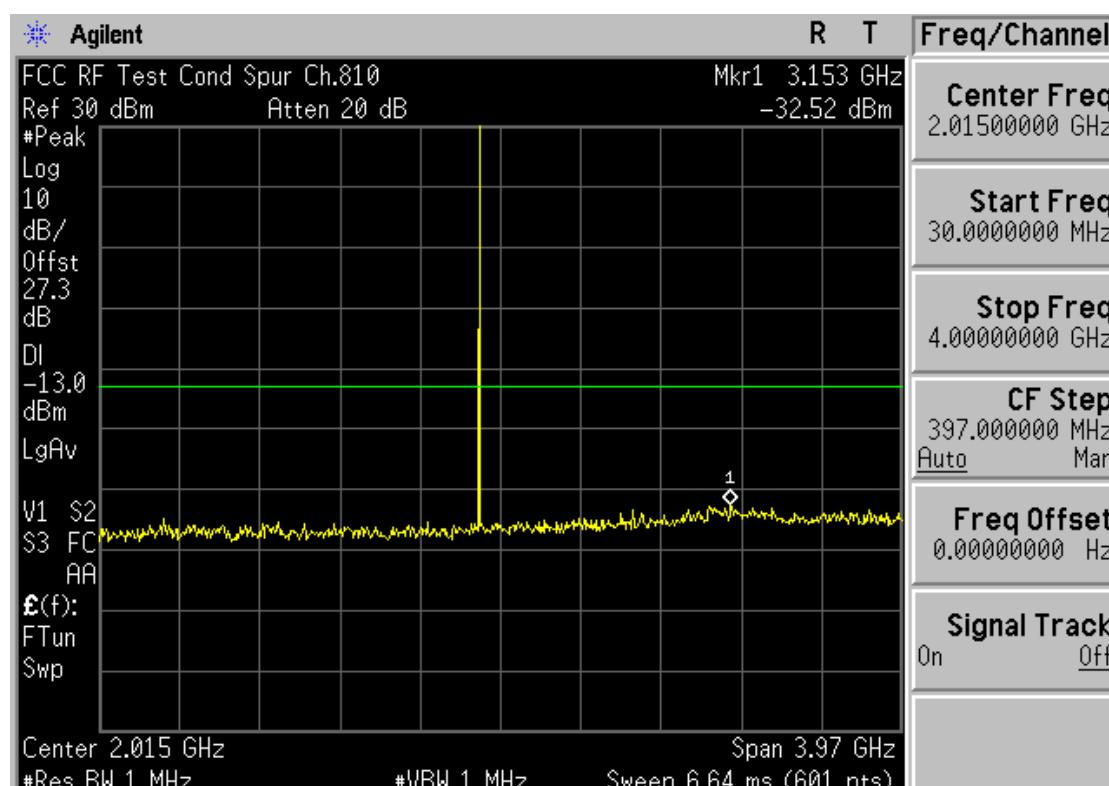
■ GSM1900 MODE (810 CH.) Conducted Spurious Emissions2
