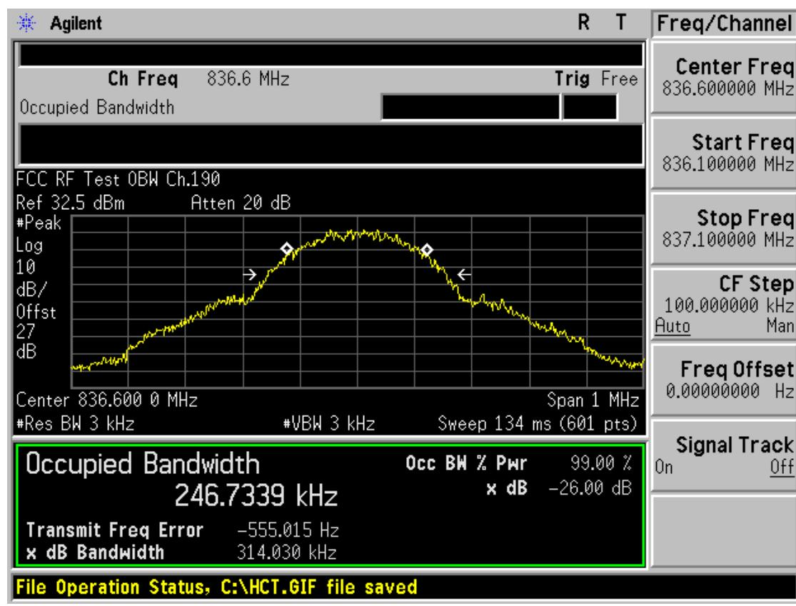
■ GSM850 MODE (251 CH.) Occupied Bandwidth
