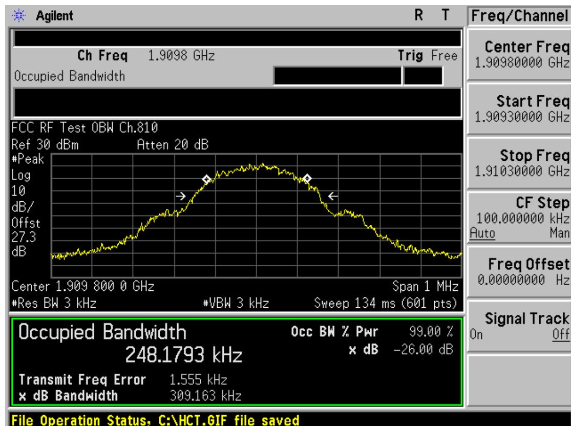
■ GSM1900 EDGE (810 CH.) Occupied Bandwidth
