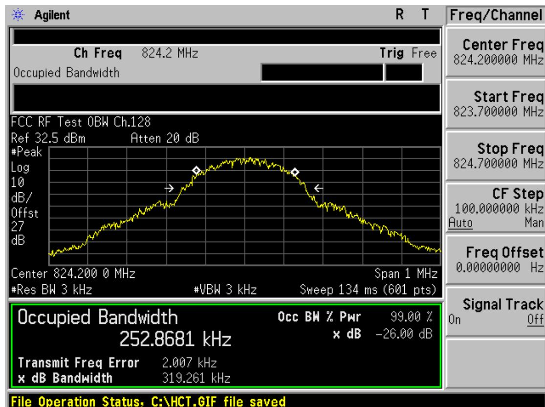
■ GSM850 MODE (190 CH.) Occupied Bandwidth
