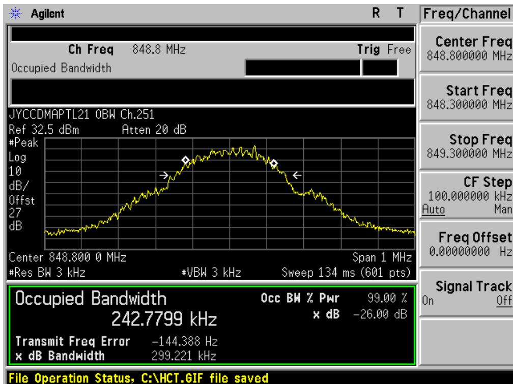
■ GSM1900 MODE (512 CH.) Occupied Bandwidth
