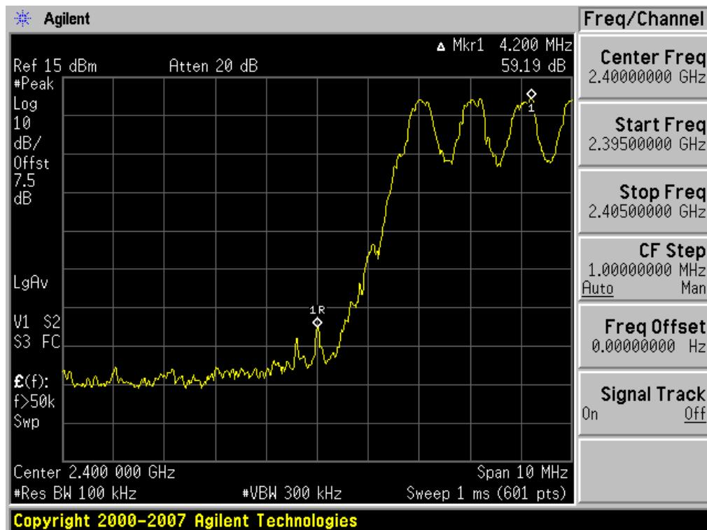
Test Plots with hopping (GFSK)
