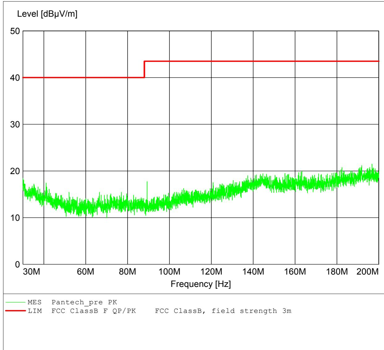
*Spurious emission under normal conditions according to FCC part 15*      Order number: G05M209010001
