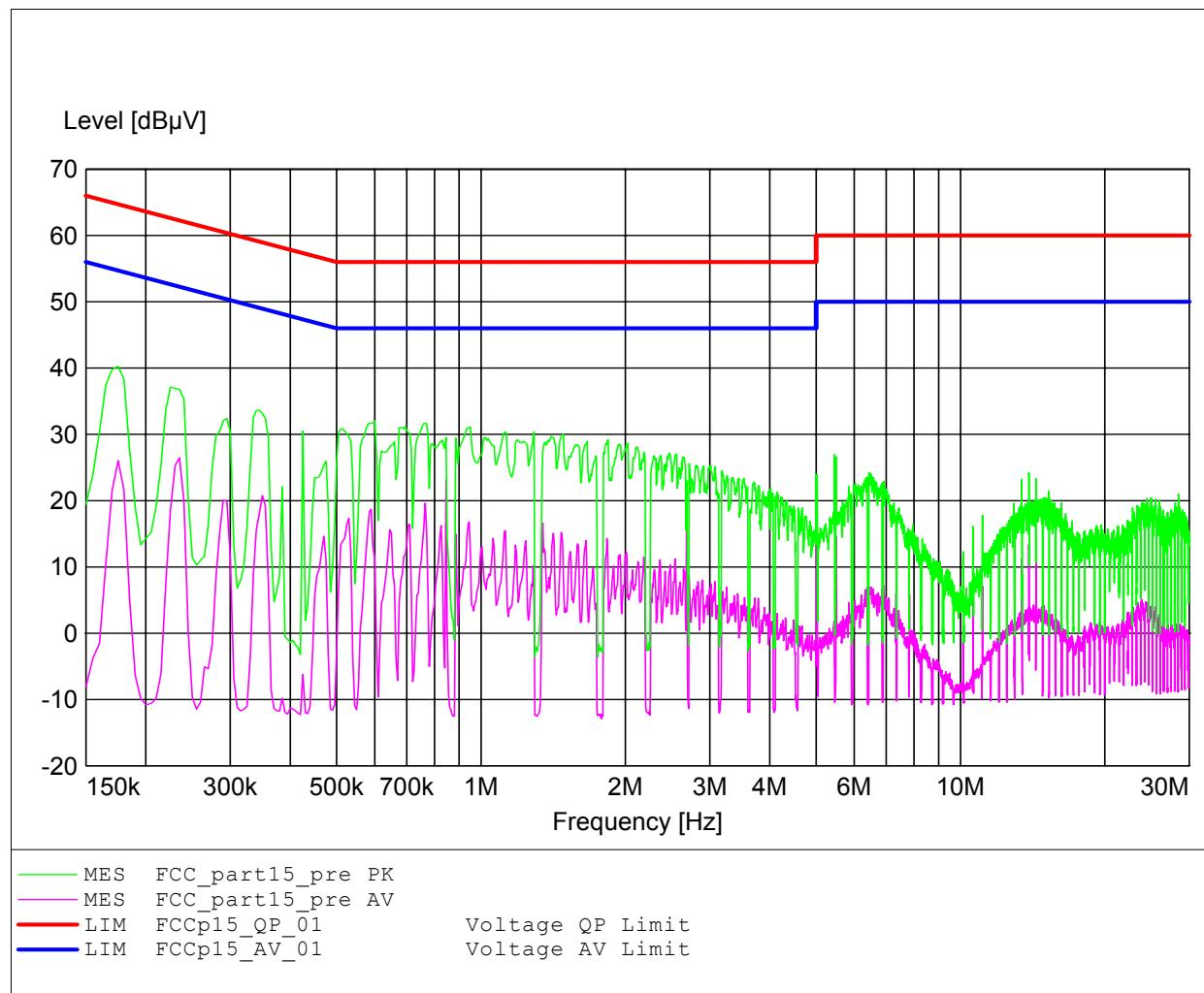
*Spurious emission under normal conditions according to FCC part 15*      Order number: G05M209010001
