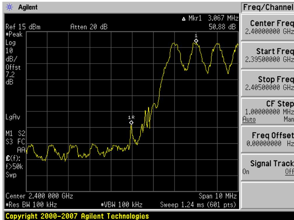
Test Plots with hopping (GFSK)
