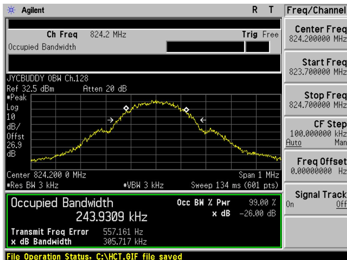
■ GSM850 MODE (190 CH.) Occupied Bandwidth
