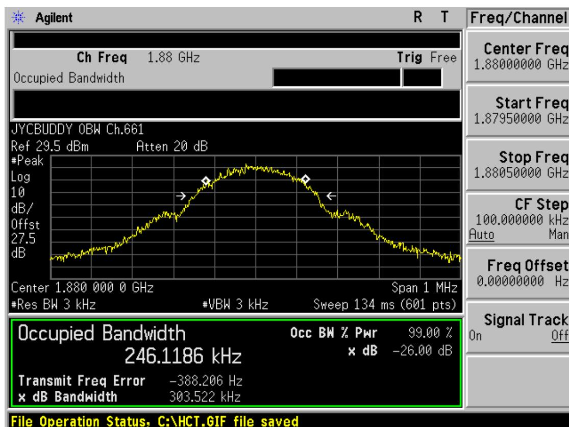
■ GSM1900 MODE (810 CH.) Occupied Bandwidth
