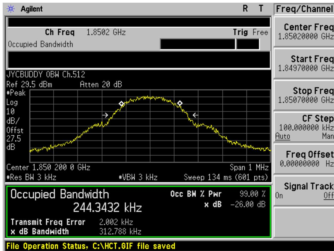
■ GSM1900 MODE (661 CH.) Occupied Bandwidth
