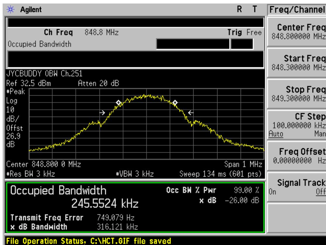
■ GSM1900 MODE (512 CH.) Occupied Bandwidth
