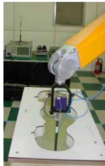
Figure 3. Photograph of the probe and the Phantom
