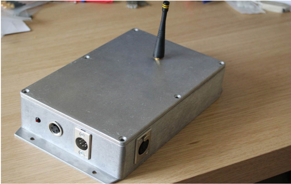
Showing the connectors and antenna The box size is approximately 222 x 146mm
