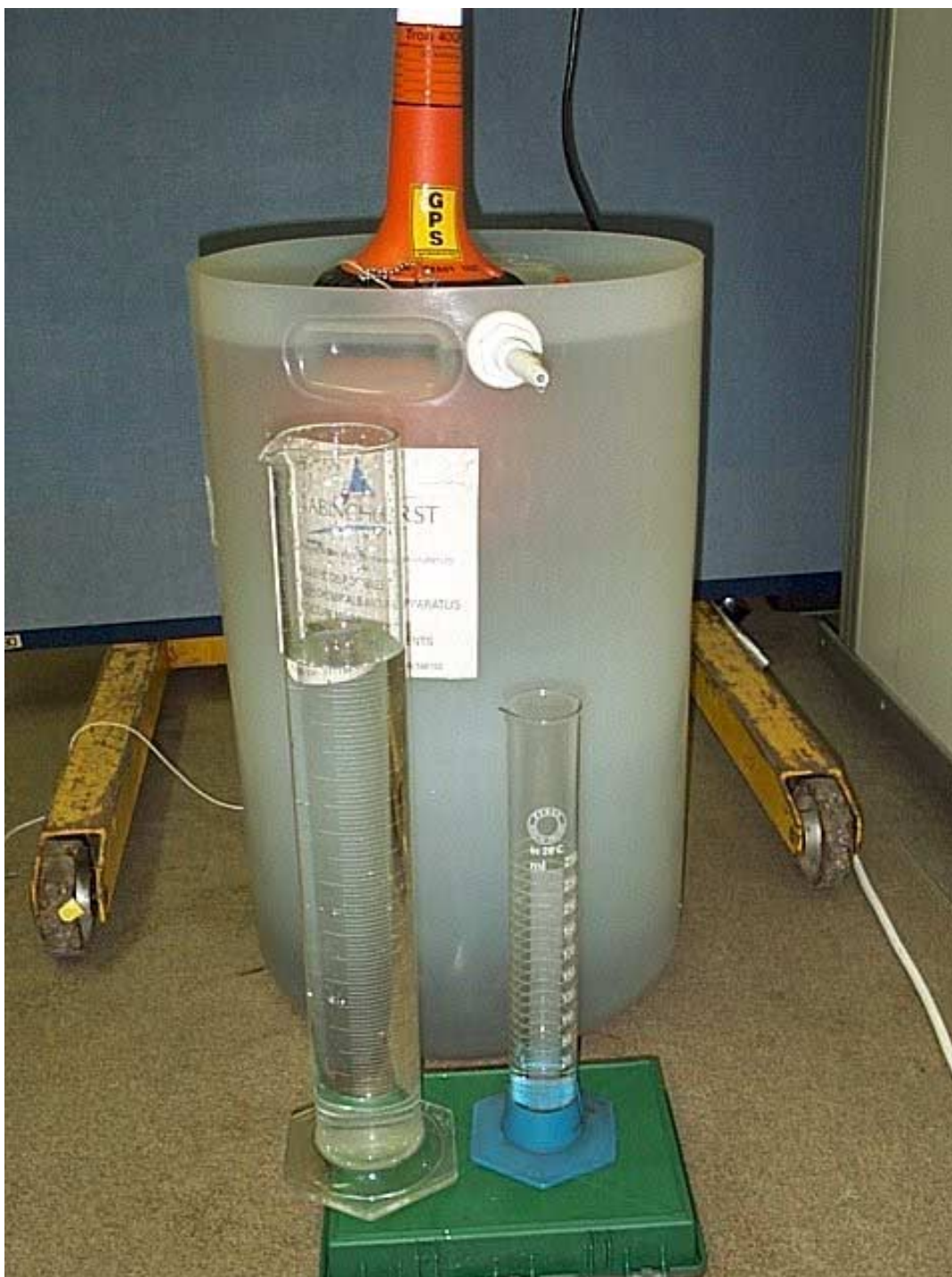
Photo 4. The set-up for testing procedure 2 – Beacon floating naturally.
