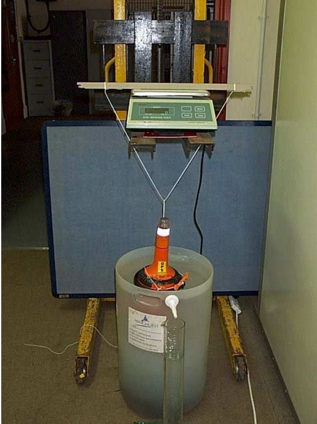
Photo 2. The set-up for testing procedure 1 – Beacon floating naturally.
