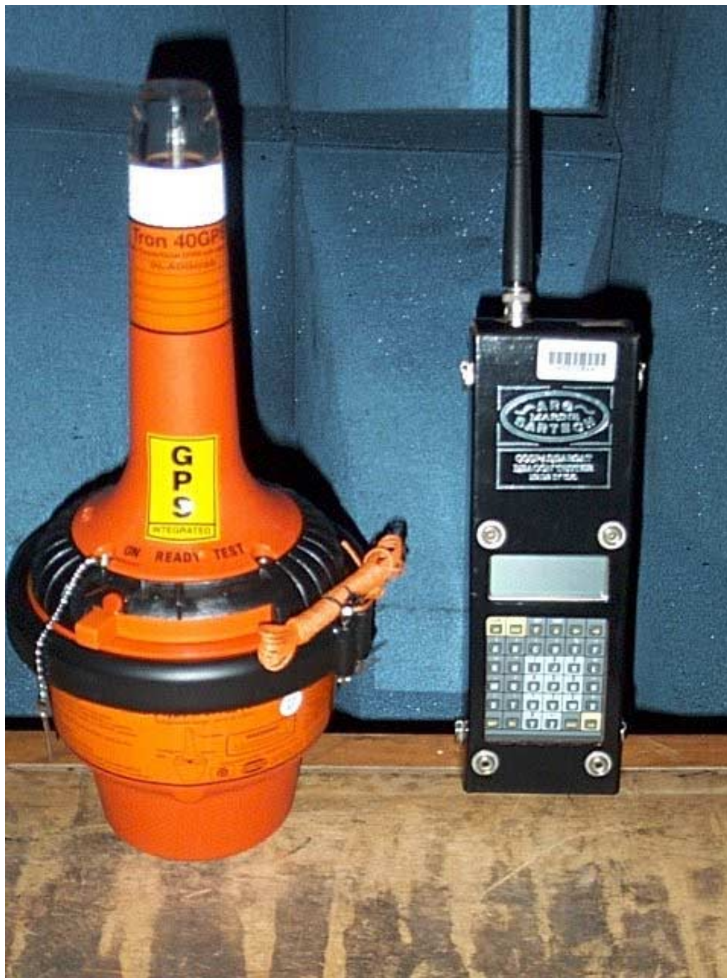
Photo 1. The TRON 40GPS Beacon and the ARG/Sartech EPIRB Tester.
