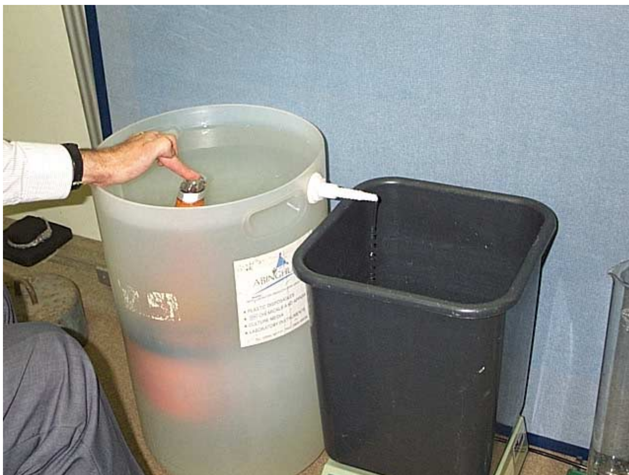
Photo 5. The set-up for testing procedure 3 – Beacon submerged.
