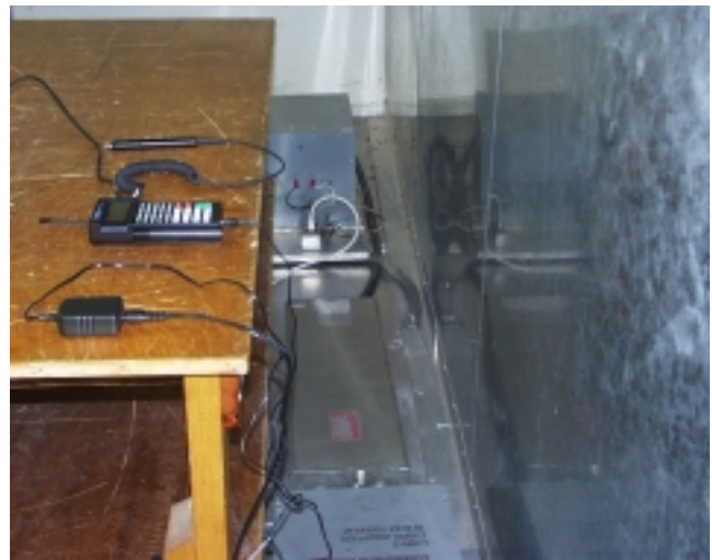
Conducted Emission Setup Photos (Worst Emission Position)
