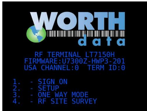
On second line on the screen, FIRMWARE: Uxxx, gives the firmware revision number. The letter U indicates USA frequency. 201 refers to the version of the radio module firmware.
