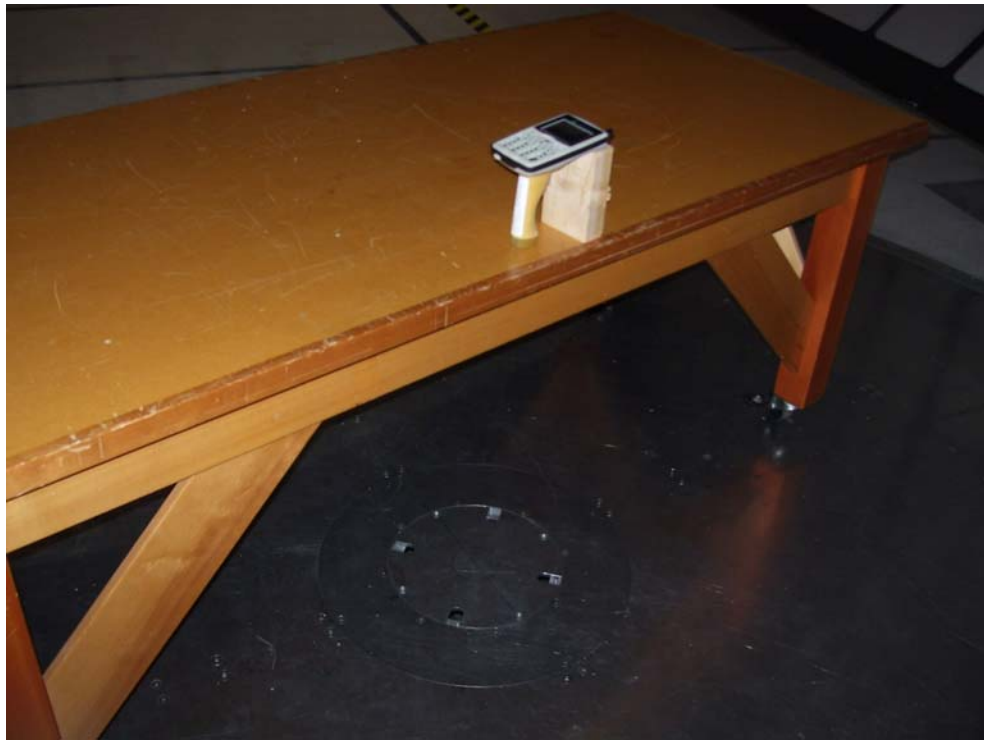
Figure 14 - Radiated Emissions Test Setup
