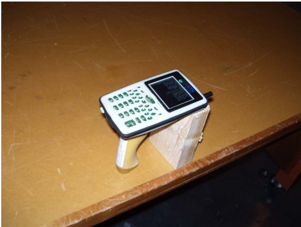
Figure 15 - Radiated Emissions Test Setup
