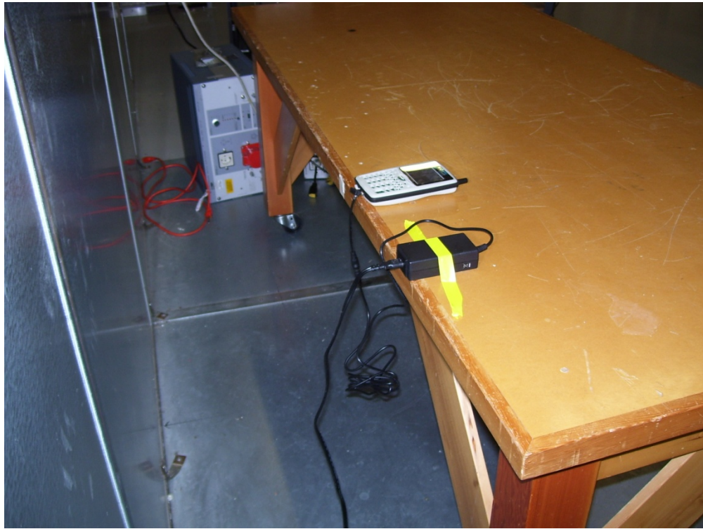
Figure 16 - Conducted Emissions Test Setup
