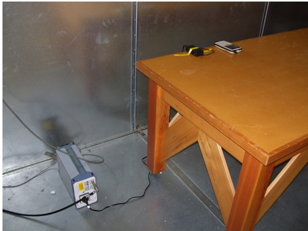
Figure 17 - Conducted Emissions Test Setup
