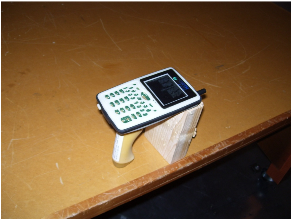
Figure 15 - Radiated Emissions Test Setup
