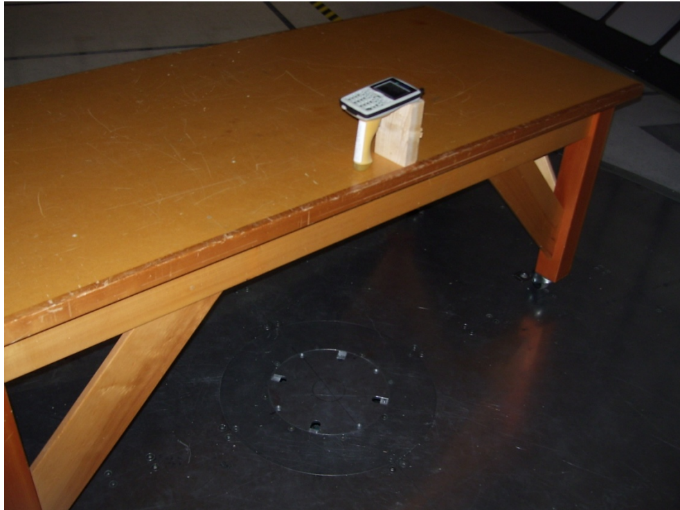
Figure 14 - Radiated Emissions Test Setup
