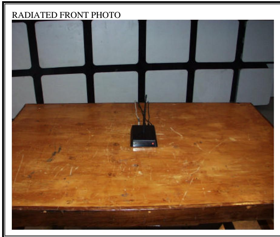
**DIGITAL DEVICE RADIATED EMISSIONS SETUP**
