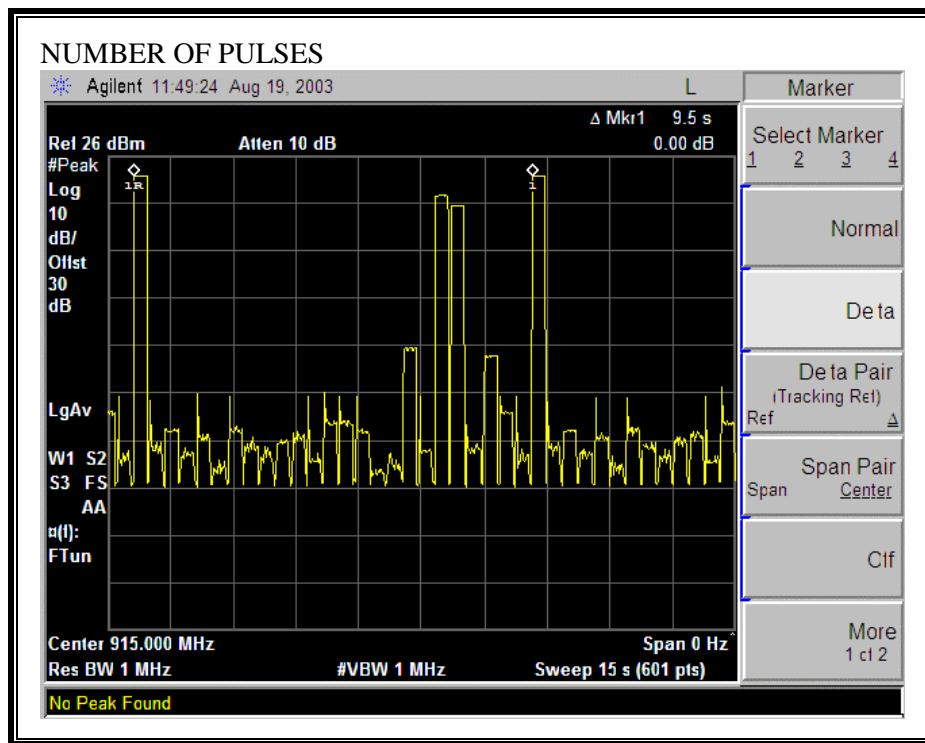
The two highest amplitude pulses occur when the channel frequency equals 915MHz. The lower amplitude pulses occur when the channel frequency is not equal to 915MHz. The amplitude of channel frequencies other than 915MHz will be a function of the delta frequency ( $F_{\text{channel}} - 915$ ) and the fall-off of the 1MHz RBW filter in the spectrum analyzer.
