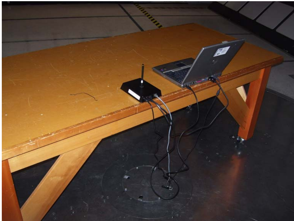
Figure 13 - Radiated Emissions Test Setup
