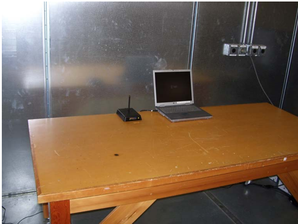
Figure 15 - Conducted Emissions Test Setup
