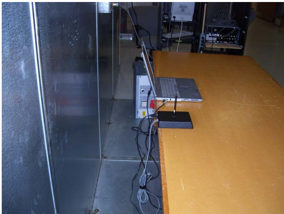
Figure 16 - Conducted Emissions Test Setup
