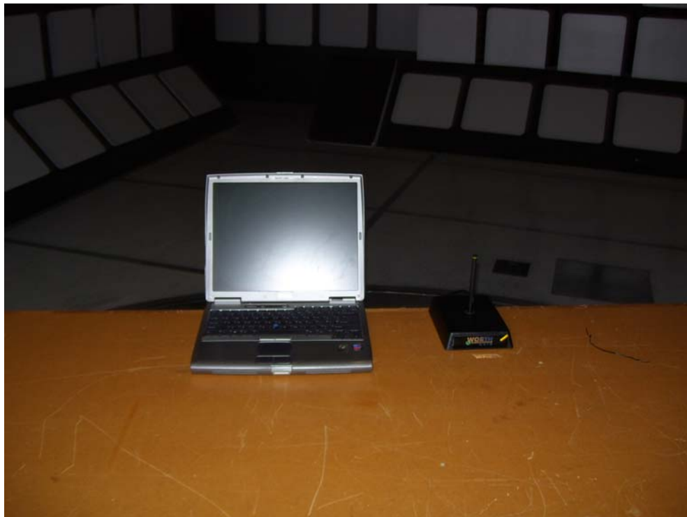
Figure 14 - Radiated Emissions Test Setup
