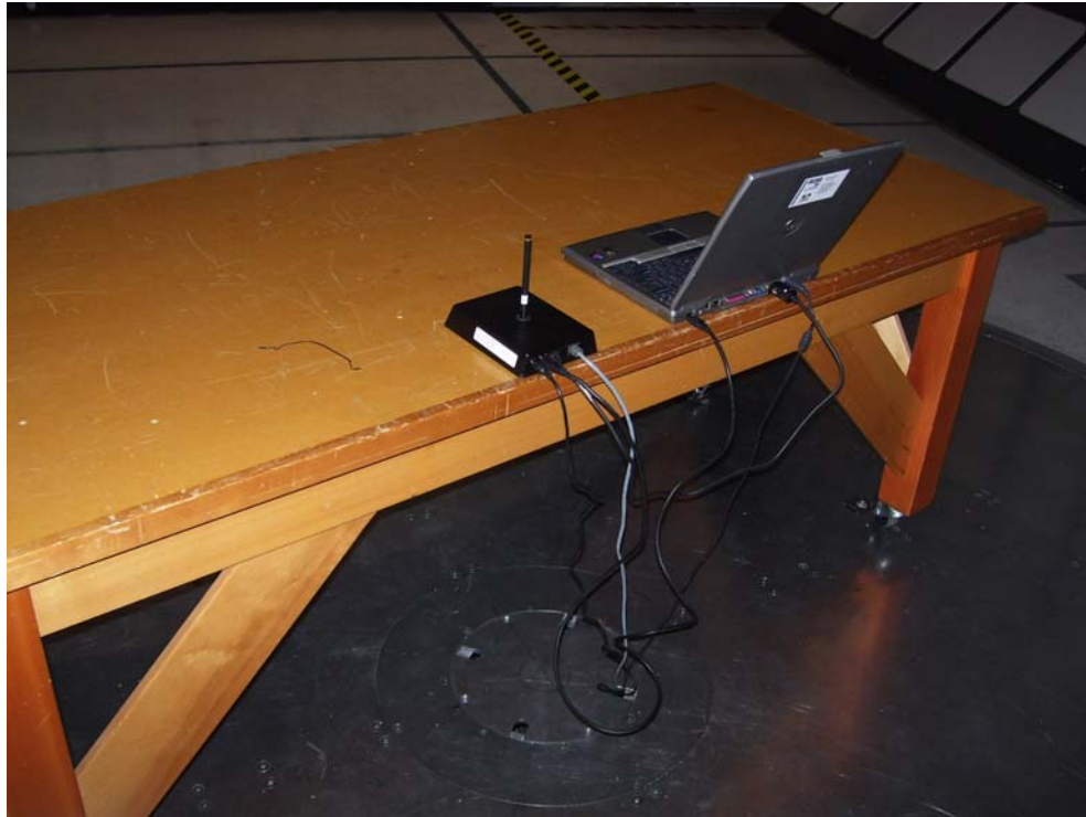
Figure 13 - Radiated Emissions Test Setup
