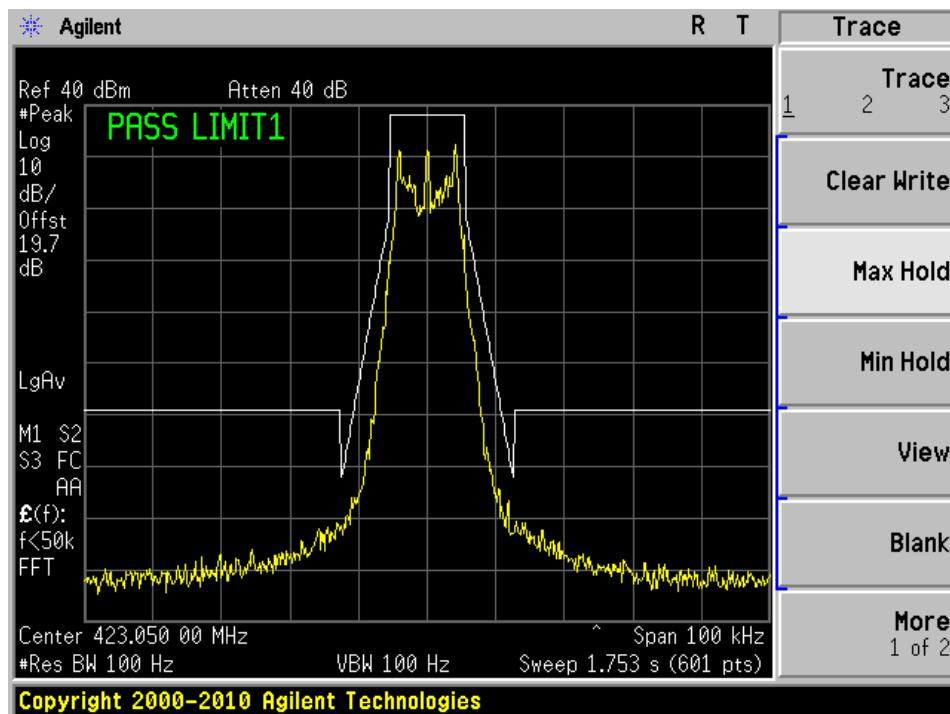
Modulation: GMSK with BT = 0.5, Data Rate: 8400 bps
