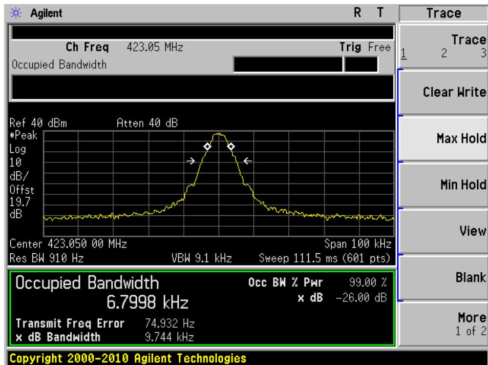
Modulation: GMSK with BT = 0.5, Data Rate: 4000 bps
