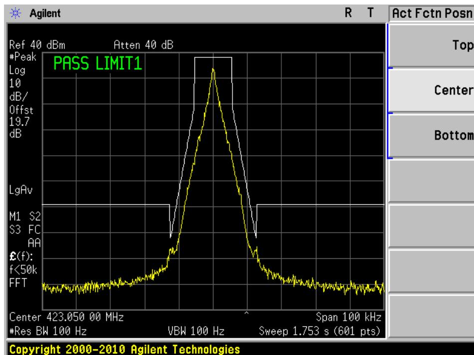
Modulation: GMSK with BT = 0.3, Channel Baud Rate: 4000 bps
