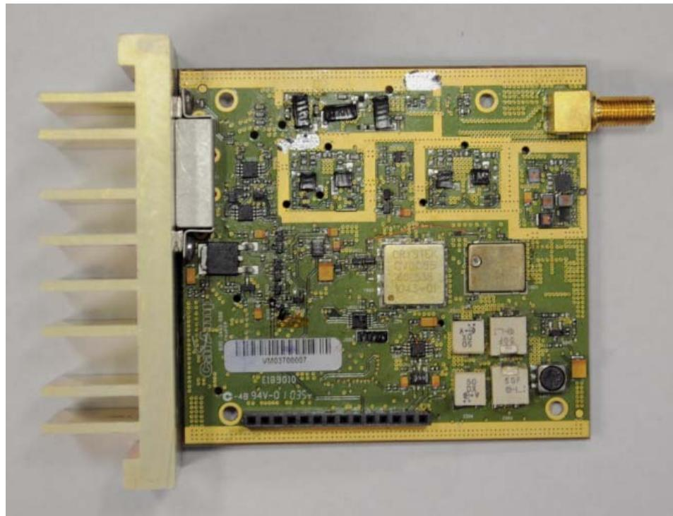
**14.11 EUT – Radio PCB (Shielding off) Bottom View**
