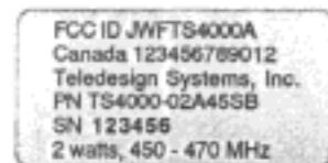
Type Acceptance Information for TS4000 Radio Modem with 3474 Transceiver
