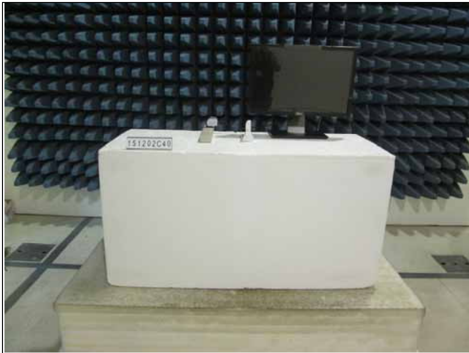
Radiated Emission Test above 1GHz
