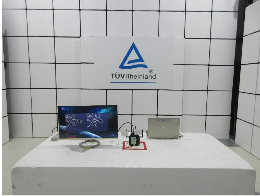
Photograph 2: Test Setup for Spurious Emissions (Front View 2)
