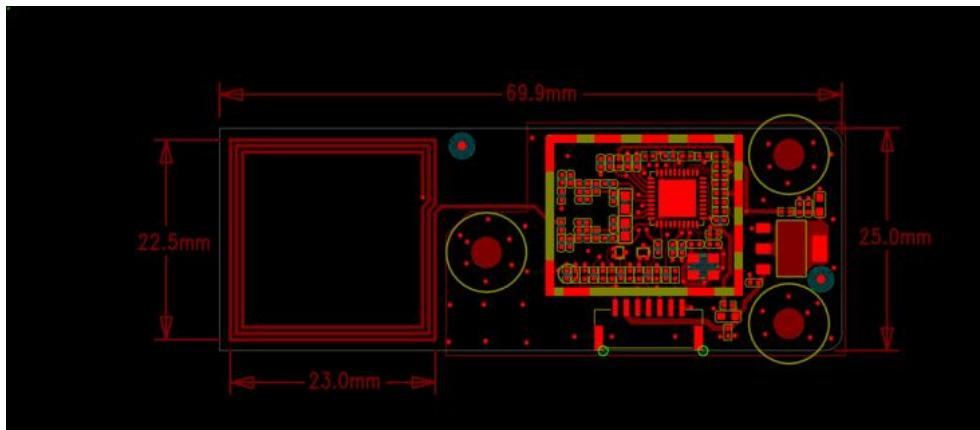
An Antenna Coil is the Coil itself, which is essentially an inductive Coil
