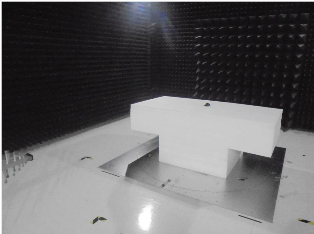
**Radiated Emission Below 1GHz Test (Charge Mode)**
