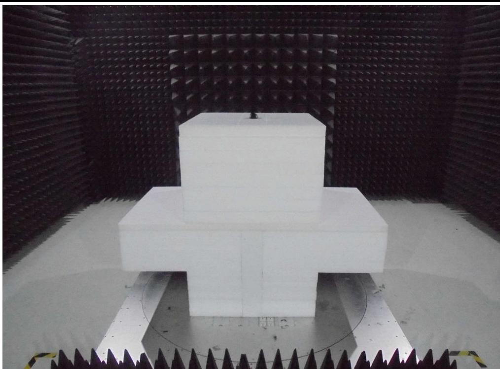
**Radiated Emission Above 1GHz Test**
