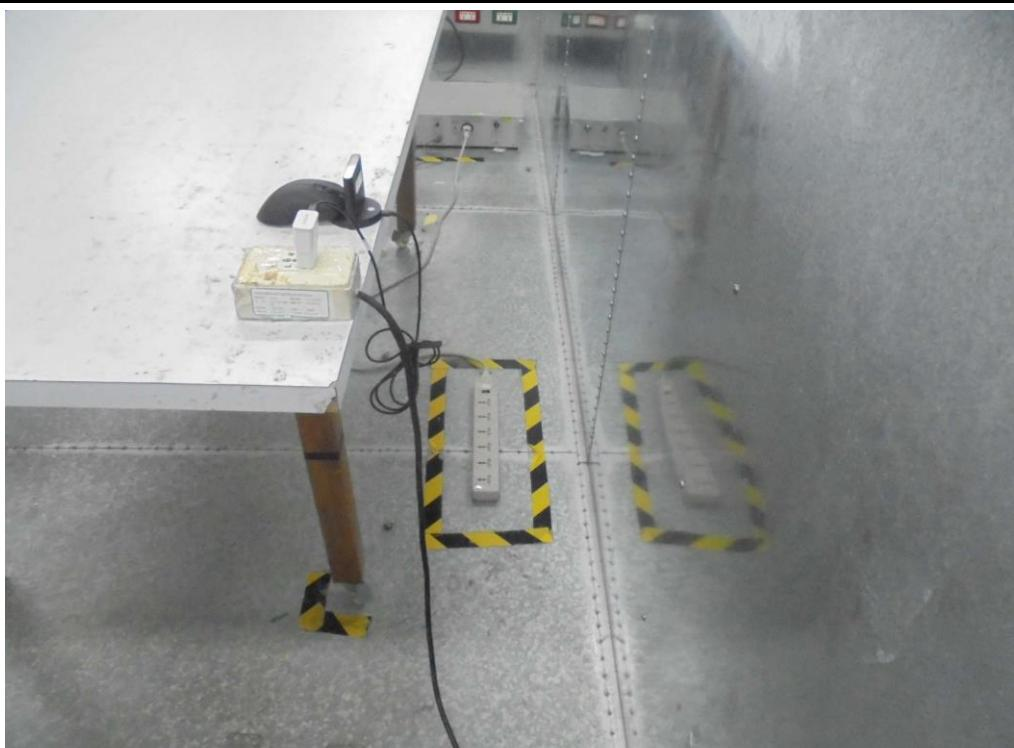
**Radiated Emission Below 1GHz Test (Battery Mode)**
