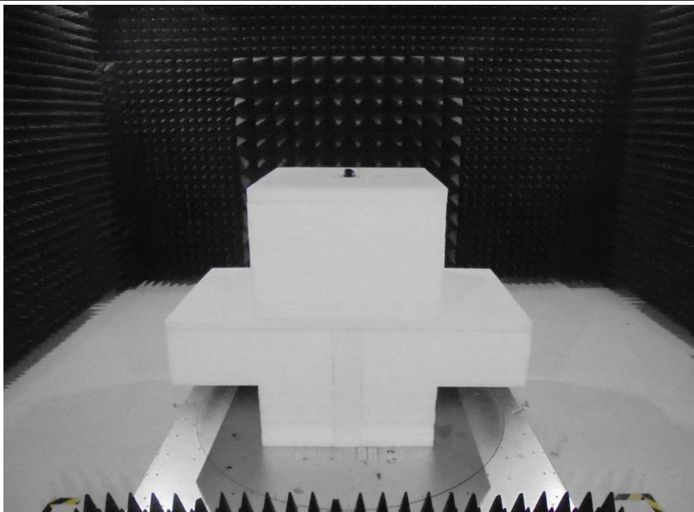
**Radiated Emission Above 1GHz Test**
