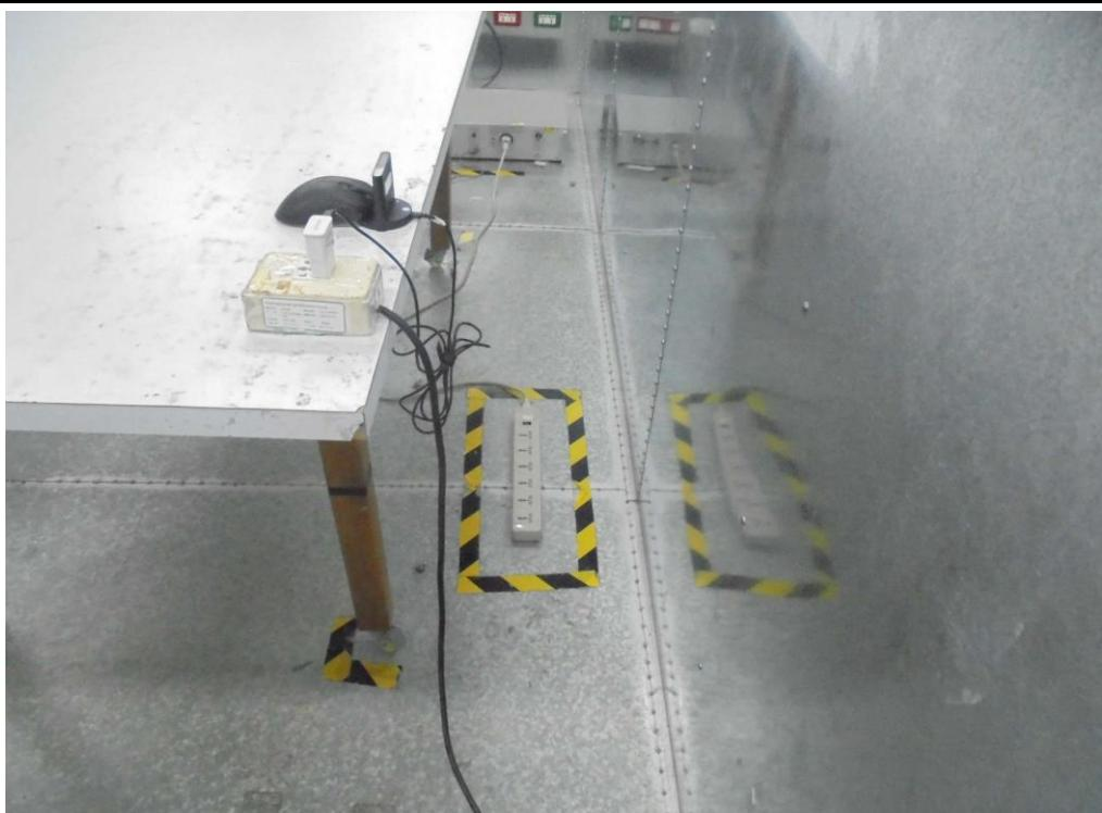
**Radiated Emission Below 1GHz Test (Battery Mode)**
