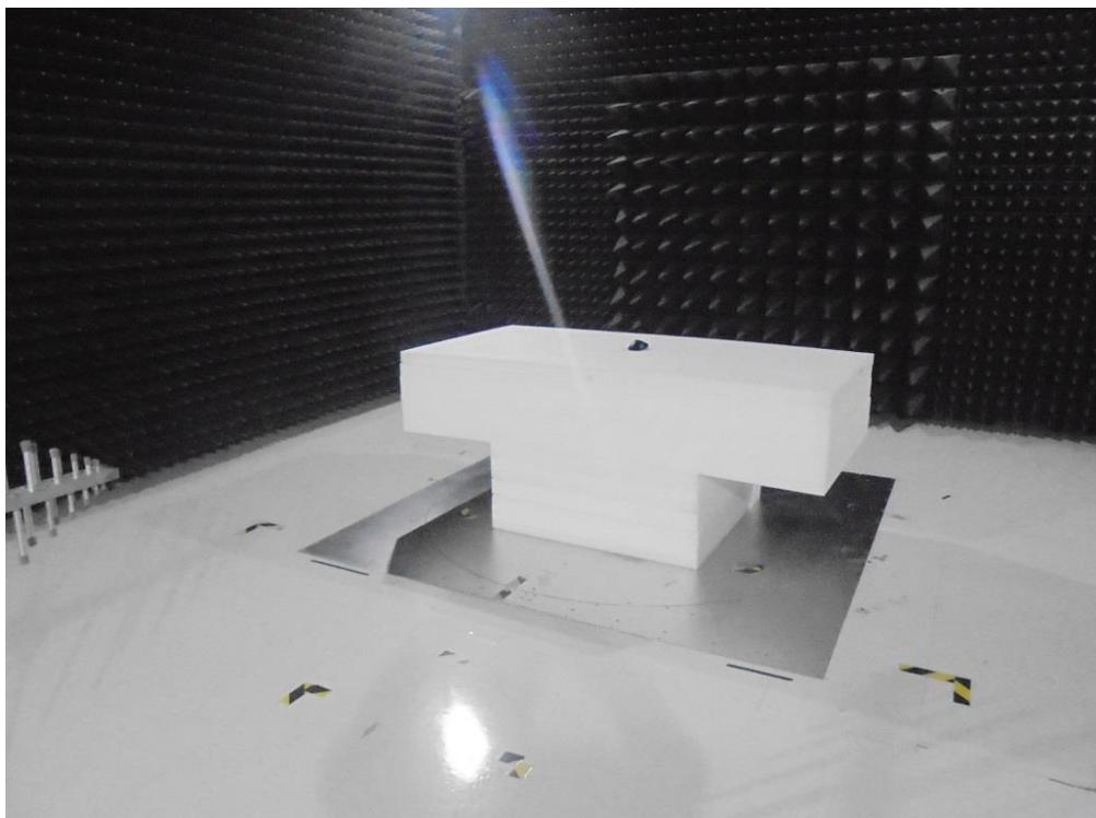
**Radiated Emission Below 1GHz Test (Charge Mode)**
