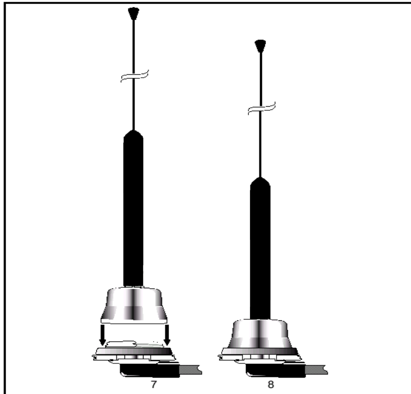
Figure 2.19 Attaching the Bulkhead Mount 850/1900 Cellular Antenna
