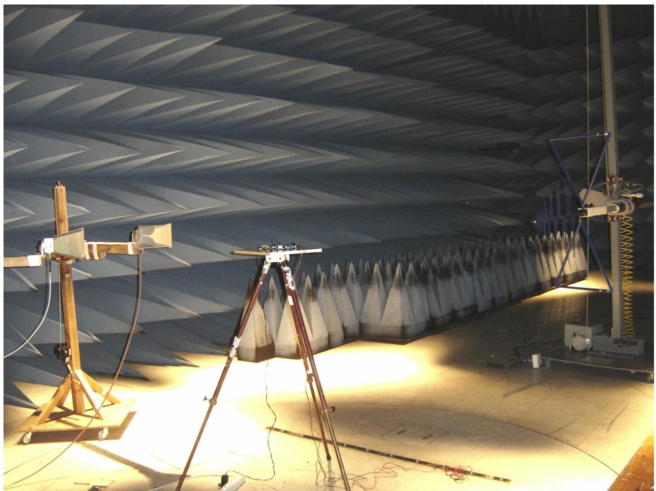
5. Test set-up for radiated measurements below 1 GHz.
