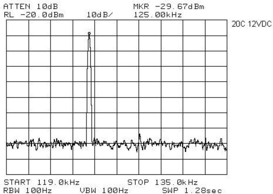
**Section 3. Radiated Emissions****Para. No.: 15.209****Test Performed By:** Russell Grant**Date of Test:** August 17, 2001**Minimum Standard:**
