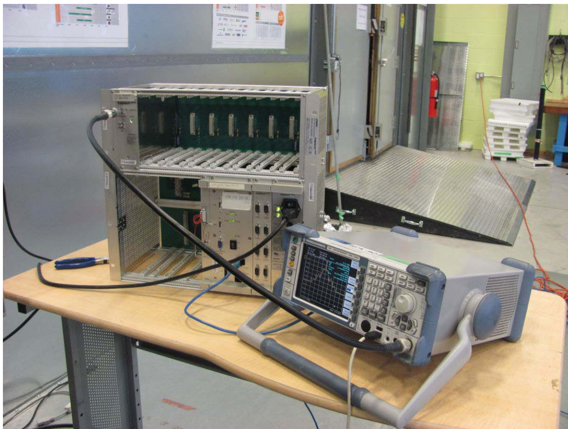
Illustration 4: Antenna conducted emission setup
