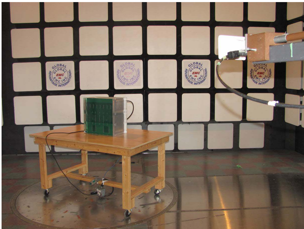
Illustration 2: 802356 Radiated emission setup - photo 2
