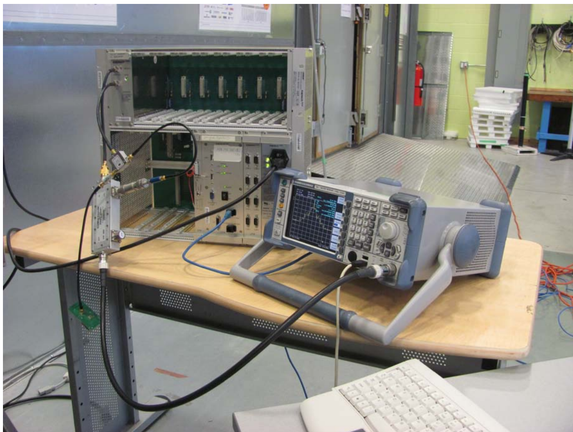
Illustration 5: Antenna conducted emission – KTDM setup with circulator
