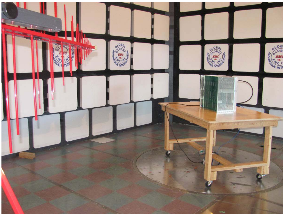
Illustration 1: 802356 Radiated emission setup – photo 1
