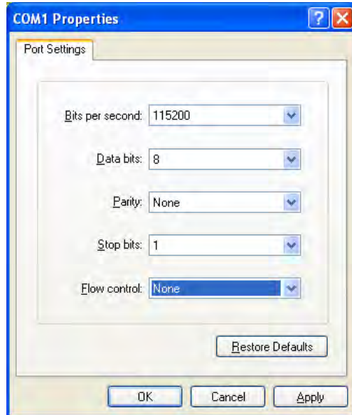
Figure 8-2: HyperTerminal Configuration for a serial connection to the Diagnostic port
