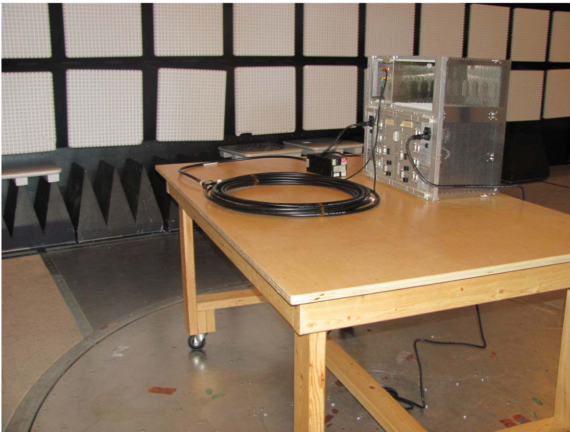
Illustration 5: 802356 Radiated emission setup – photo 1
