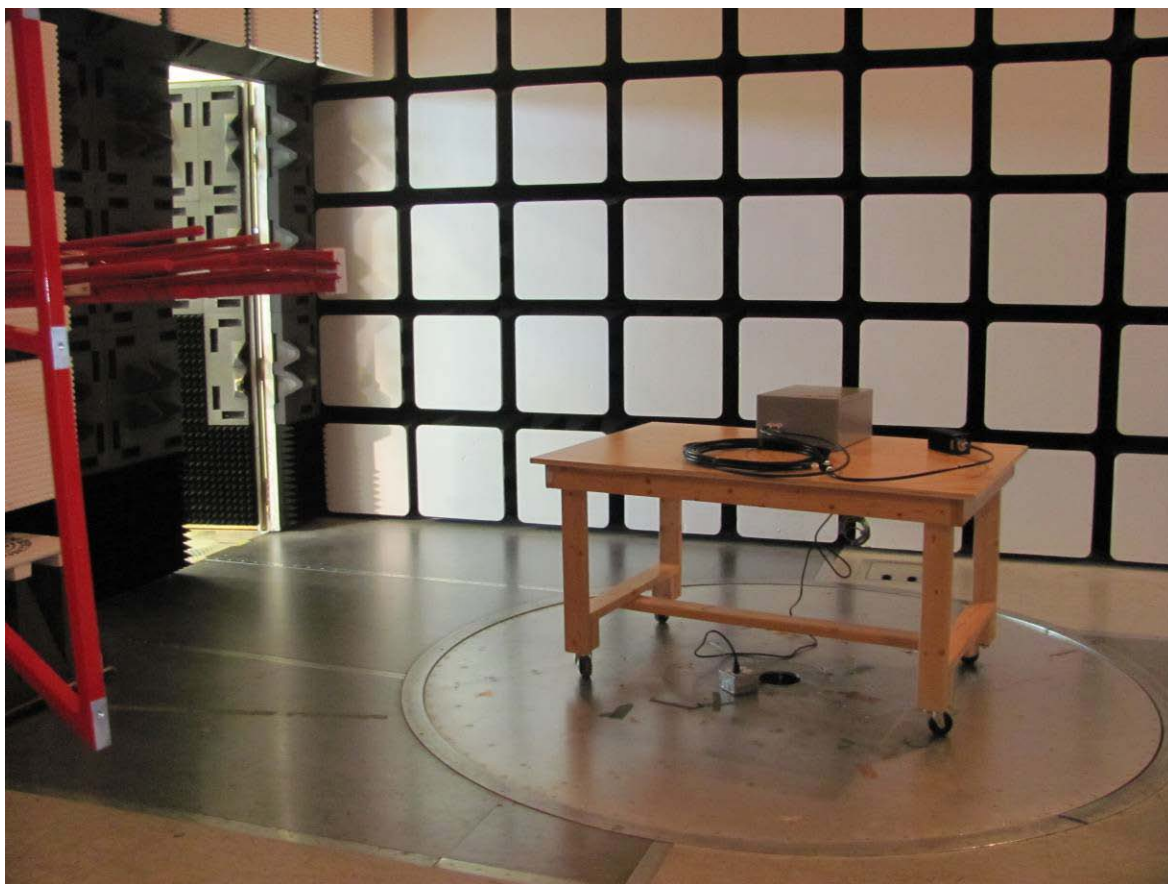
Illustration 12: 802356 Radiated emission setup – photo 2
