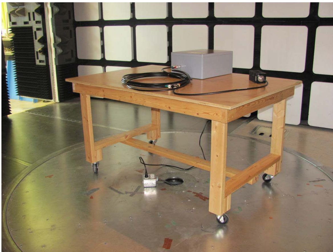
Illustration 11: 802356 Radiated emission setup – photo 1
