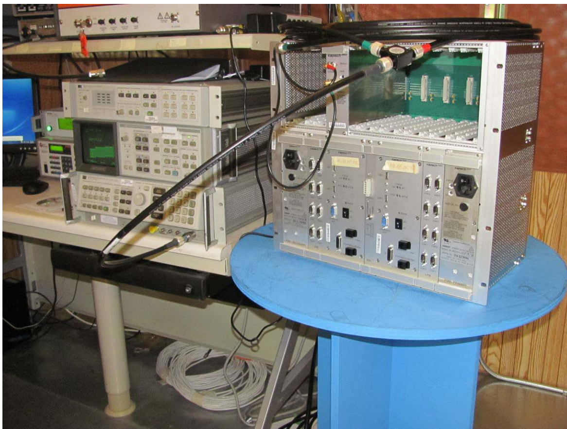
Illustration 8: Antenna conducted emission setup
