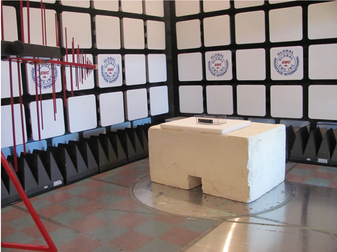
Illustration 3: Radiated emission setup – photo 1
