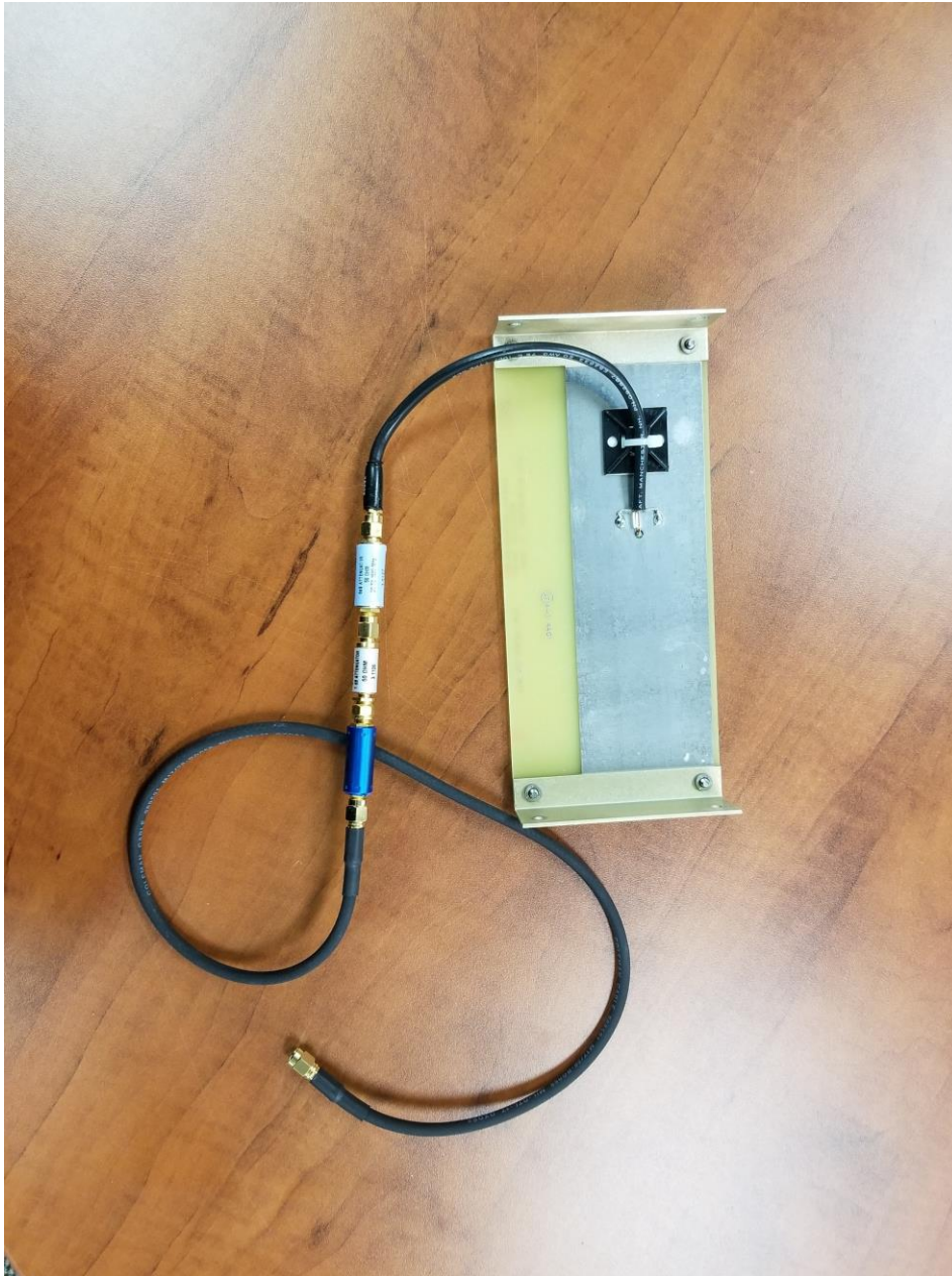
Tag Programmer/Tester T500/T600 Basic Unit Model 800890 Patch Antenna Assembly – Top Photo
