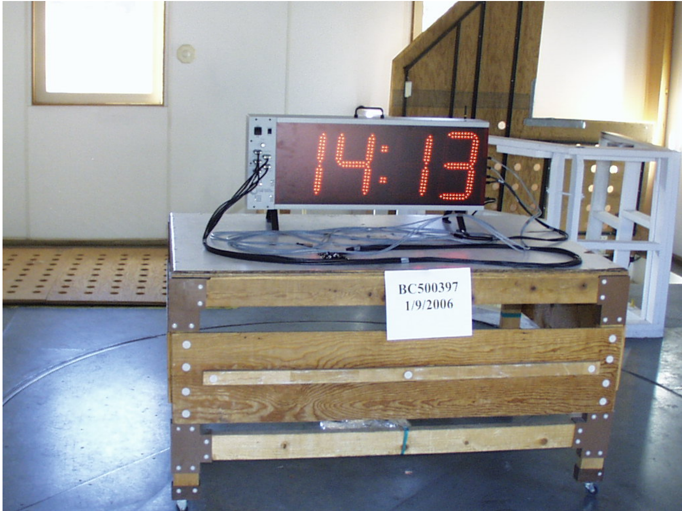
Test-setup photo(s): Radiated Unintentional Emissions:
