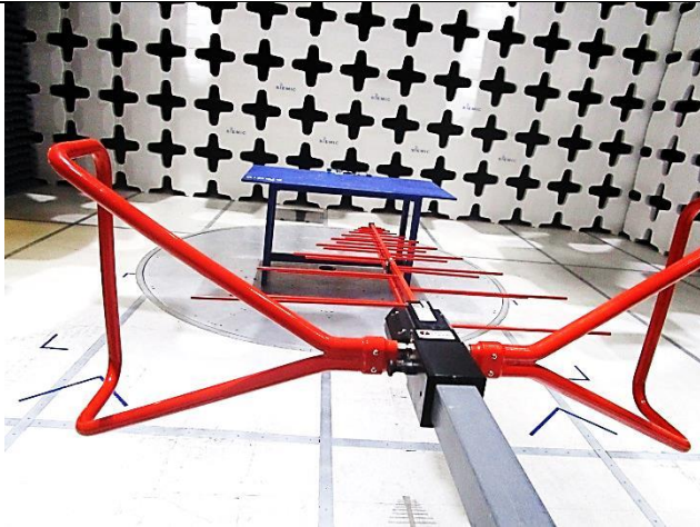
Radiated Emissions (<1GHz) – Front View
