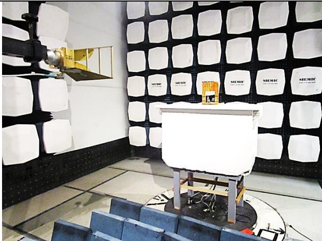
Radiated Emissions (>1GHz) – Front View
