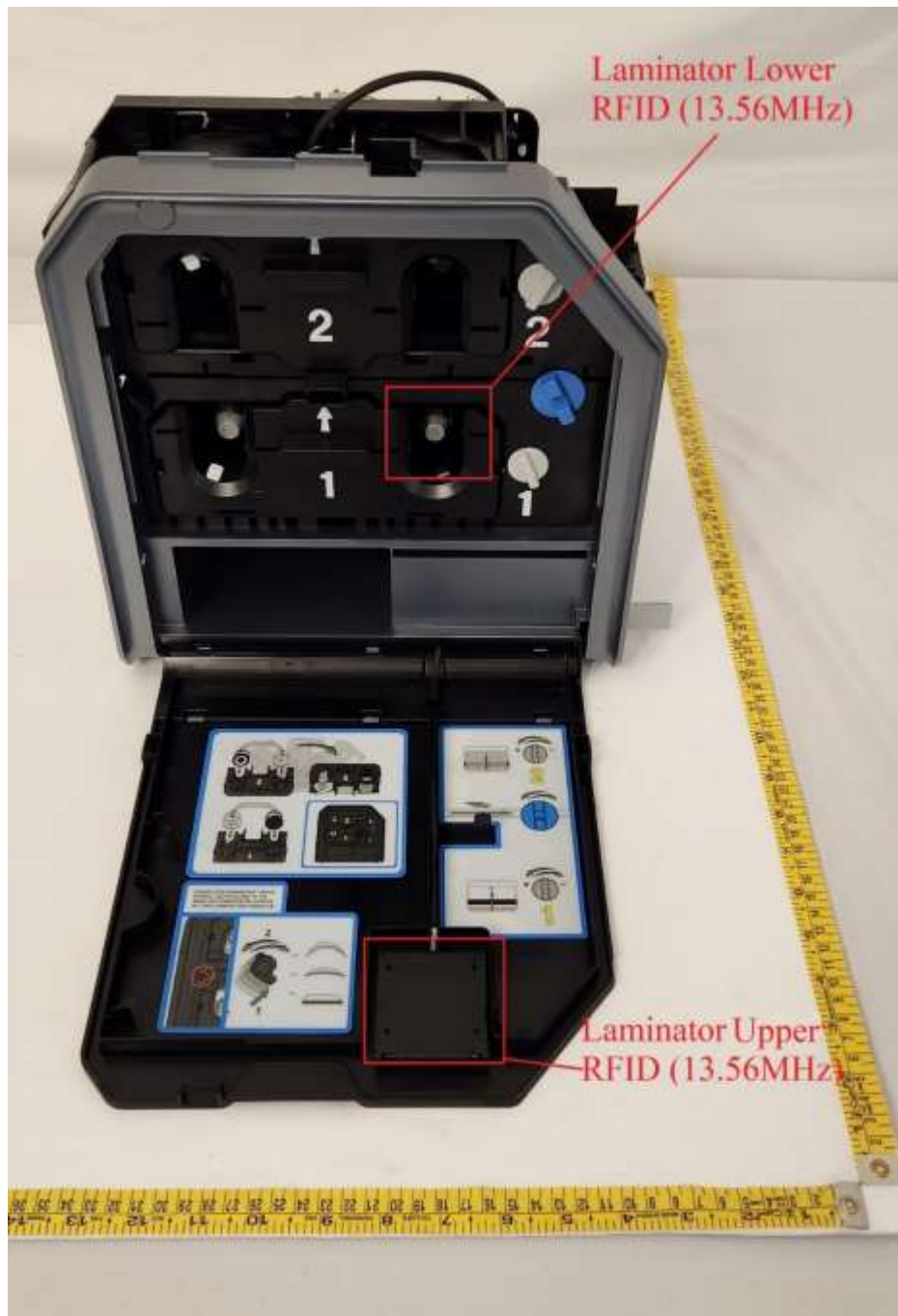
Laminator Upper/Lower RFID Antenna Location
