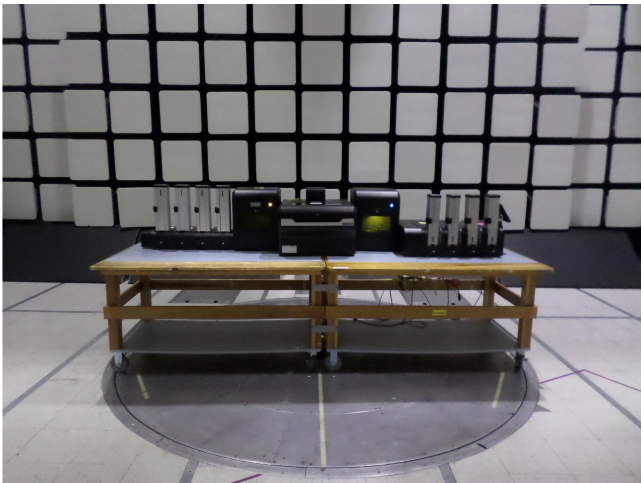
Figure 10: Radiated Spurious Emissions - 30-1000 MHz, Front View
