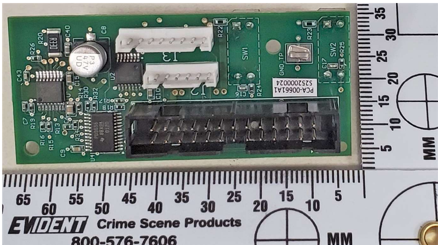
Input Hopper Controller Board Top Side
